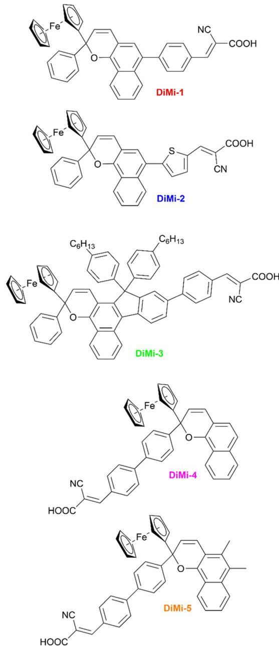
**Scheme 1** Structures of the synthesized photochromic dyes in the closed form: **DiMi-1** (with phenyl spacer); **DiMi-2** (with thiophene spacer); **DiMi-3** (with indeno bridge spacer); **DiMi-4** (with inverted structure) and **DiMi-5** (with inverted structure and methyl groups).
