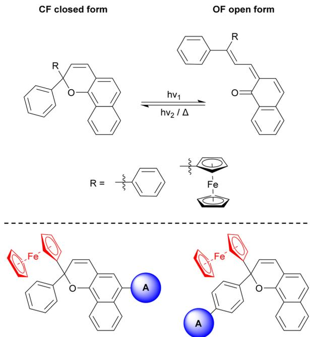
**Fig. 1** Photo-induced reversible isomerization process in diphenyl-naphthopyran molecules between the closed form (CF) and the open form (OF) the molecules with and without ferrocene modification are represented. Below, naphthopyran dyes with a ferrocene group and presenting also an acceptor moiety (A) in different geometries.
