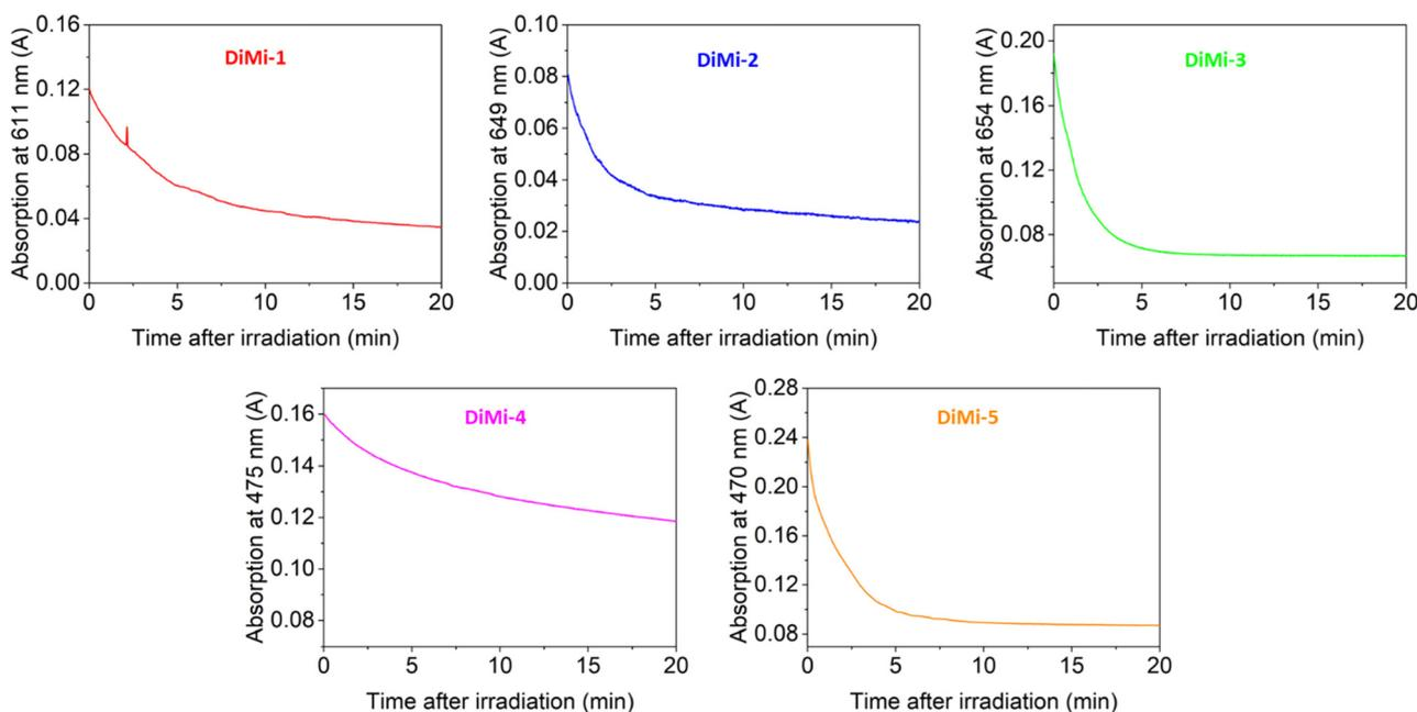
Fig. 3 Discoloration curves of the described dyes in solution ( $2 \times 10^{-5}$  M in toluene, 25 °C) in the dark after the PSS was reached under irradiation with polychromatic light. For each dye a wavelength representative of the difference between the OF and CF was monitored (611 nm) for **DiMi-1**, 649 nm for **DiMi-2**, 654 nm for **DiMi-3**, 475 nm for **DiMi-4** and 470 nm for **DiMi-5**.
