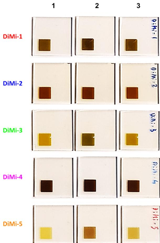
Fig. 5 TiO<sub>2</sub> electrodes grafted with the synthesized dyes. (1) Before irradiation, (2) after irradiation and (3) after five days in the dark.
