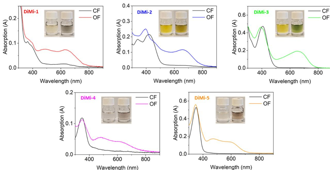
Fig. 2 UV-visible absorption spectra of the described dyes ( $2 \times 10^{-5}$  M in toluene, 25 °C) before irradiation (black curves) and after reaching the PSS with continuous irradiation with a polychromatic lamp (coloured curves).
