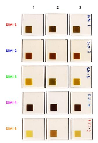
Fig. 5  $\,$  TiO $_2$  electrodes grafted with the synthesized dyes. (1) Before irradiation, (2) after irradiation and (3) after five days in the dark.
