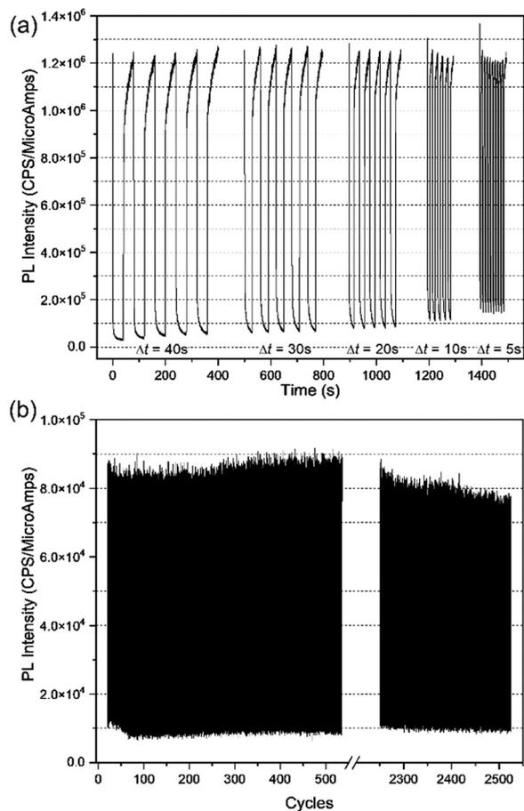
Fig. 4 (a) EFC chrono-fluorometry of p(g-DPATPE-Ph) ECD, switching at  $\pm 1.5$  V at different  $\Delta t$  of 40, 30, 20, 10, and 5 s. (b) Long-term EFC switching stability of p(g-DPATPE-Ph) ECD, with voltage alternating at  $\pm 1.5$  V at  $\Delta t$  of 20 s, for 2500 cycles.
