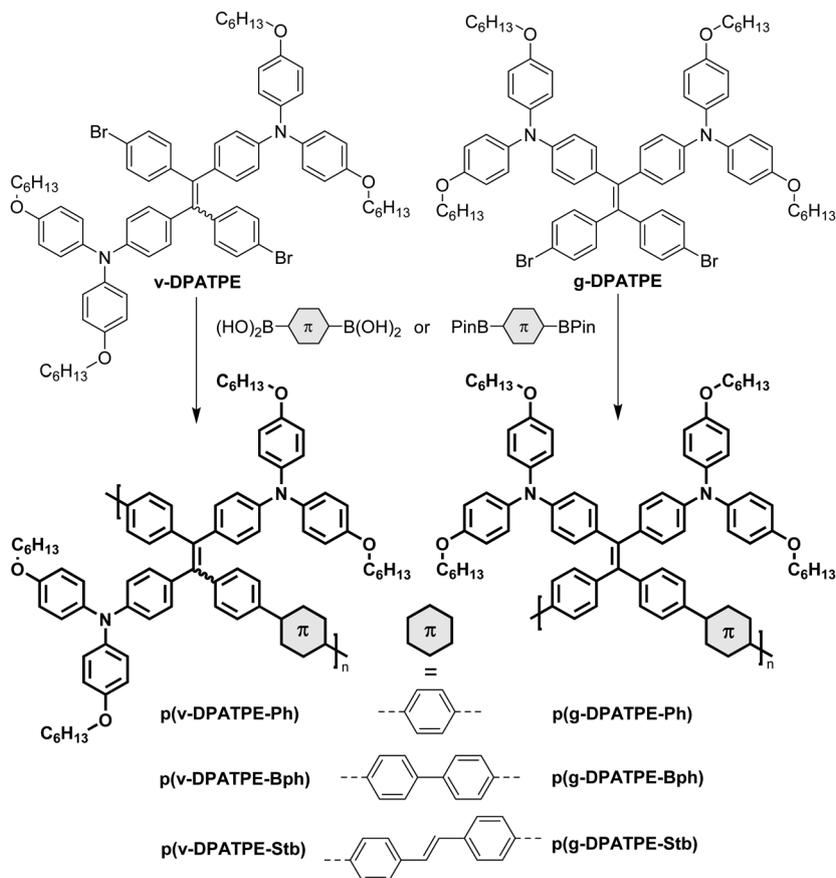
**Scheme 1** Chemical structures of novel monomers *v*-DPATPE and *g*-DPATPE, and AIE-active EFC conjugated polymers, p(*v*-DPATPE-Ph), p(*g*-DPATPE-Ph), p(*v*-DPATPE-Bph), p(*g*-DPATPE-Bph), p(*v*-DPATPE-Stb), and p(*g*-DPATPE-Stb).
