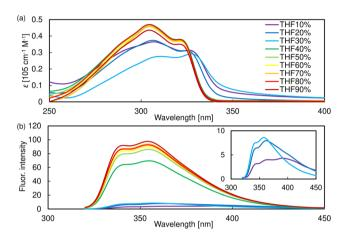
(a) Absorption and (b) fluorescence spectra of B5CT[7] in THF/ water mixed solvent at  $1.0 \times 10^{-5}$  M.
