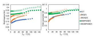
Fig. 7 (a)  $\Delta n$  and (b)  $\Delta S$  of **5CT** ( $\bullet$ ), **B5Q[7]** ( $\triangle$ ), **B5OQ[7]** ( $\triangle$ ), **B5BPhEB[7]** (■), and **B5OBPhEB[7]** (□) at each  $T_{IN} - T$ .
