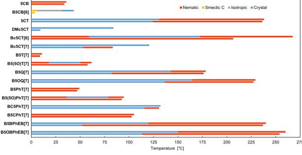
Fig. 3 Schematic diagram showing the phase transition temperatures and ranges of the compounds, except for B5CB[7], B8CB[7], B7OCB[7], and B5CT[7]; upper bar: upon heating, lower bar: upon cooling
