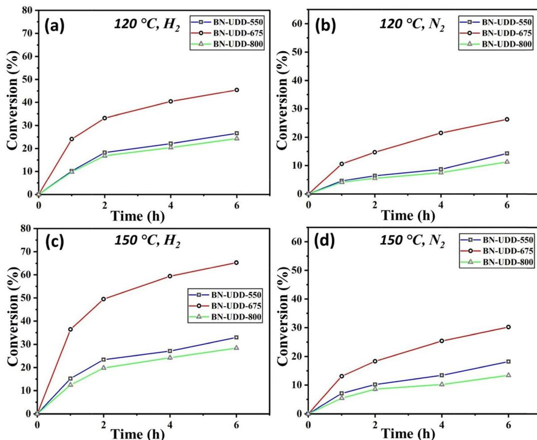
**Fig. 1** Conversion vs. time graphs of different catalysts at (a) 120 °C under H<sub>2</sub> gas, (b) 120 °C under N<sub>2</sub> gas, (c) 150 °C under H<sub>2</sub> gas, and (d) 150 °C under N<sub>2</sub> gas.
