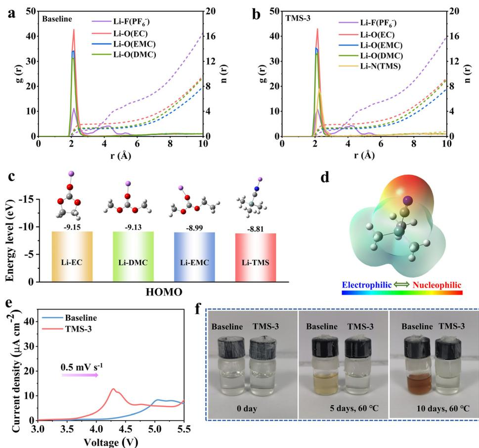
**Fig. 1** Radial distribution function  $g(r)$  and coordination number  $n(r)$  of  $\text{Li}^+$  calculated from MD simulations in the (a) baseline and (b) TMS-containing electrolytes. (c) Theoretical calculations of HOMO values for solvents and additive solvated with  $\text{Li}^+$ . (d) ESP charge distribution of TMS. (e) LSV tests at a scan rate of  $0.5 \text{ mV s}^{-1}$ . (f) High-temperature storage tests for the baseline and TMS-3 electrolytes at  $60^\circ\text{C}$ .
