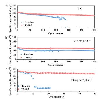
Fig. 4 Cycling performance with different electrolytes under various conditions at 2-4.8 V: (a) at 3C; (b) at 0.33C and -15 °C; (c) at 0.5C with a high mass loading of 13 mg cm<sup>-2</sup>.
