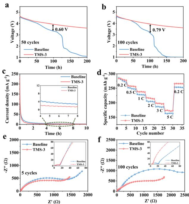
**Fig. 3** (a) and (b) Self-discharge curves of Li||LRM batteries using different electrolytes at 4.8 V after (a) 50 and (b) 100 cycles. (c) Constant voltage floating charge test at 4.8 V in different electrolytes after 100 cycles. (d) Rate performance. (e) and (f) Nyquist plots of Li||LRM batteries in baseline and TMS-3 electrolytes after (e) 5 and (f) 100 cycles.
