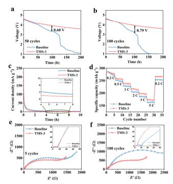
Fig. 3 (a) and (b) Self-discharge curves of LillLRM batteries using different electrolytes at 4.8 V after (a) 50 and (b) 100 cycles. (c) Constant voltage floating charge test at 4.8 V in different electrolytes after 100 cycles. (d) Rate performance. (e) and (f) Nyquist plots of Li||LRM batteries in baseline and TMS-3 electrolytes after (e) 5 and (f) 100 cycles.
