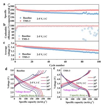
Fig. 5 Cycling performance of batteries with the two electrolytes at 2-5 V: (a) discharge capacity curves; (b) CE; (c) average discharge voltage; (d) and (e) charge and discharge curves (d) without and (e) with TMS.
