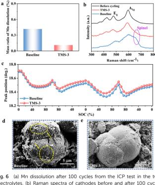
Fig. 6 (a) Mn dissolution after 100 cycles from the ICP test in the two electrolytes. (b) Raman spectra of cathodes before and after 100 cycles with different electrolytes. (c) In situ evolution of the (003) peak during the first two cycles at 0.5C. (d) and (e) SEM images of the cycled cathodes in the (d) baseline and (e) TMS-3 electrolytes.
