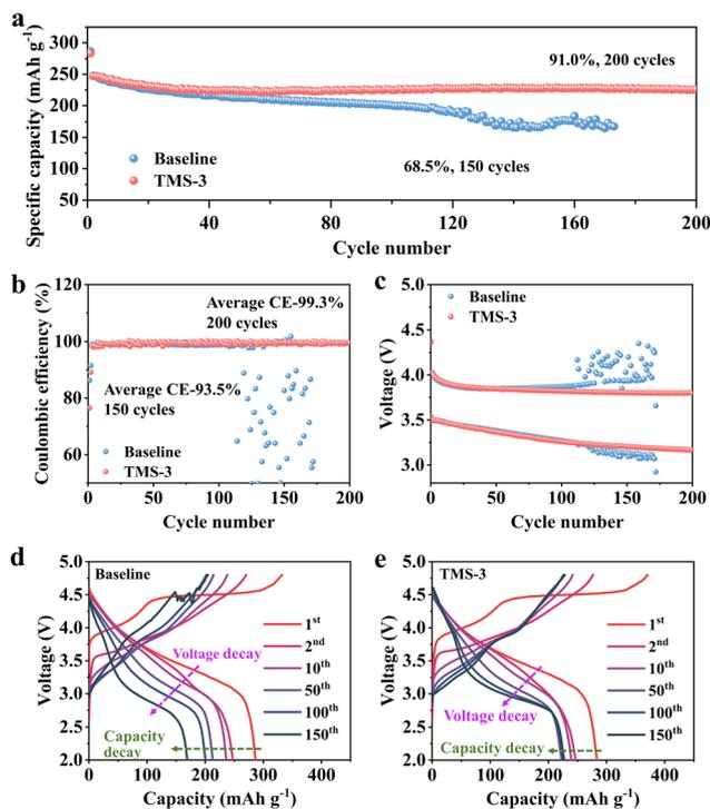
**Fig. 2** (a) Cycling performance of Li||LRM batteries with the baseline and TMS-containing electrolytes between 2 and 4.8 V at 1C. (b) The comparison of coulombic efficiency in the two electrolytes. (c) Average charge and discharge voltages during cycling. (d) and (e) Charge and discharge curves of Li||LRM batteries (d) without and (e) with TMS.
