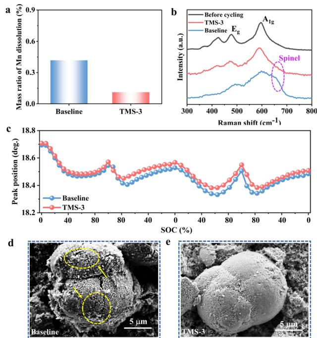
**Fig. 6** (a) Mn dissolution after 100 cycles from the ICP test in the two electrolytes. (b) Raman spectra of cathodes before and after 100 cycles with different electrolytes. (c) *In situ* evolution of the (003) peak during the first two cycles at 0.5C. (d) and (e) SEM images of the cycled cathodes in the (d) baseline and (e) TMS-3 electrolytes.
