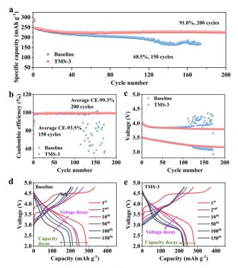
Fig. 2 (a) Cycling performance of Li|LRM batteries with the baseline and TMS-containing electrolytes between 2 and 4.8 V at 1C. (b) The comparison of coulombic efficiency in the two electrolytes. (c) Average charge and discharge voltages during cycling. (d) and (e) Charge and discharge curves of LillLRM batteries (d) without and (e) with TMS.
