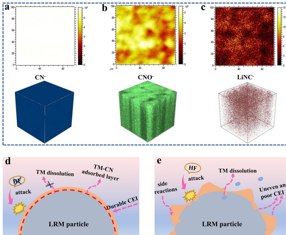
**Fig. 8** (a)–(c) TOF-SIMS 2D and 3D render images of fragments on the cycled cathodes with the TMS-3 electrolyte: (a)  $\text{CN}^-$  (as shown on the adjacent ruler, bright white color represents a high content); (b)  $\text{CNO}^-$ ; (c)  $\text{LiNC}^-$ ; (d) and (e) schematic illustrations of the performance improvement mechanism by (d) the baseline electrolyte and (e) the TMS-3 electrolyte.
