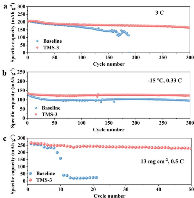
Fig. 4 Cycling performance with different electrolytes under various conditions at 2–4.8 V: (a) at 3C; (b) at 0.33C and  $-15\text{ }^{\circ}\text{C}$ ; (c) at 0.5C with a high mass loading of  $13\text{ mg cm}^{-2}$ .
