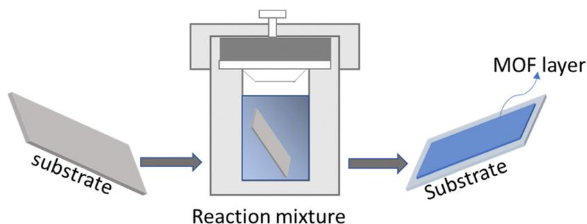
Fig. 8 MOF-based electrode construction by direct solvothermal growth.
