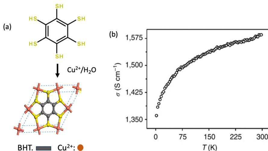
Fig. 3 (a) Electrically conductive Cu-BHT 2D MOFs designed by  $\pi$ -conjugation (b) electrical conductivity measurement of Cu-BHT film as a function of temperature ranging from 2 to 300 K. Reproduced with permission from Zhu *et al.*<sup>36</sup> Copyright Springer Nature, 2015.
