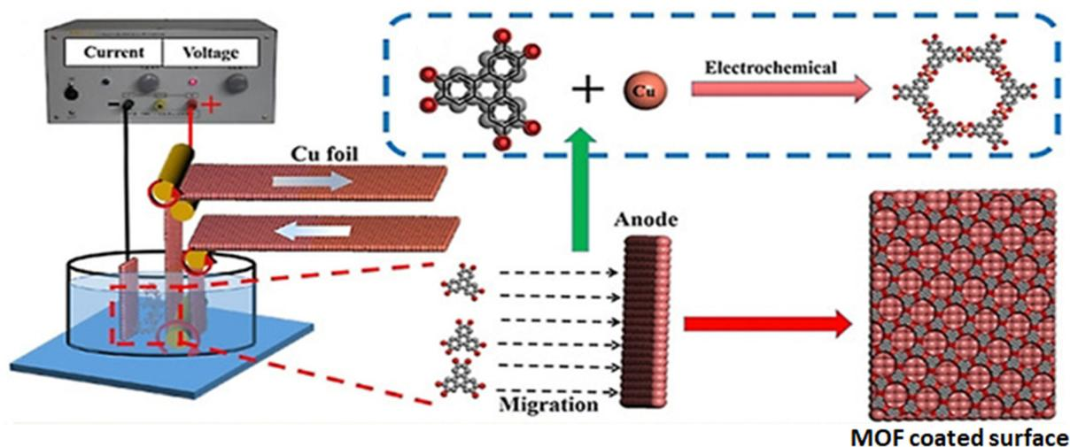
Fig. 10 MOF-based electrode construction by electrophoretic deposition. Reproduced from Liu *et al.*<sup>128</sup> Copyright 2021, Wiley-VCH.
