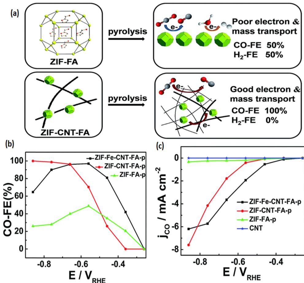
Fig. 19 (a) Schematic showing the pyrolysis of ZIFs on multi-walled carbon nanotubes (MWCNT) which aid interparticle conductivity and enhance the mass transport in  $\text{CO}_2\text{RR}$ . (b)  $\text{FE}_{\text{CO}}$  and (d) partial CO current for different catalysts at different applied potentials. Reproduced with permission from Guo *et al.*<sup>168</sup> Copyright 2017, Royal Society of Chemistry.
