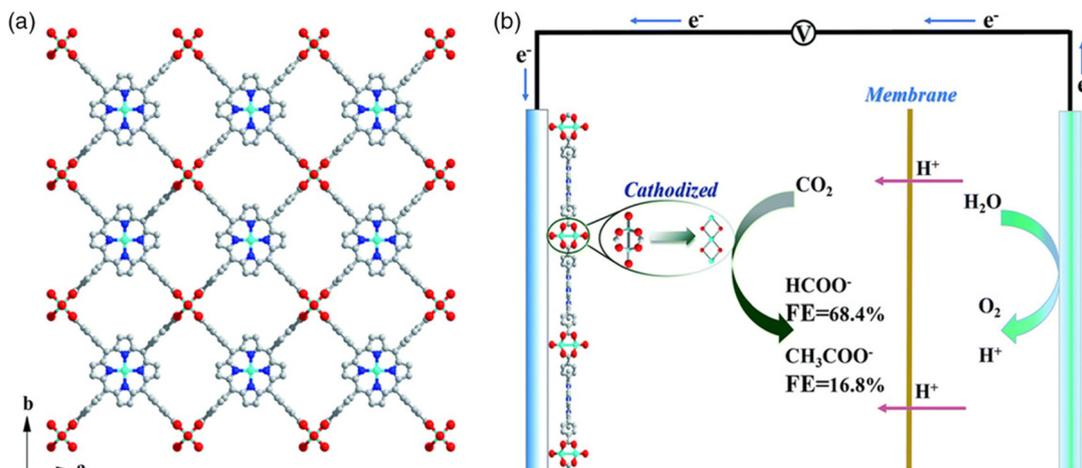
Fig. 14 (a) Crystal structure of  $\text{Cu}_2(\text{CuTCPP})$  MOF nanosheets; (b) schematic of electrochemical system showing electrocatalytic reduction of  $\text{CO}_2$  on  $\text{Cu}_2(\text{CuTCPP})$  nanosheets. Reproduced with permission from Wu *et al.*<sup>100</sup> Copyright 2019, Royal Society of Chemistry.
