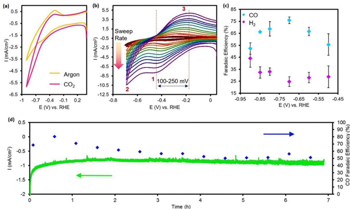
Fig. 13 (a) CV scan of the  $\text{Al}_2(\text{OH})_2\text{TCPP-Co}$  MOF catalyst showing a current increase in a  $\text{CO}_2$  environment relative to an argon-saturated environment. (b) Varying scan rate with corresponding redox potentials (c) plot of the faradaic efficiency at the potential range of  $-0.5$  to  $0.9$  V vs. RHE; (d) MOF stability test with corresponding FE measurement. Reproduced from Kornienko *et al.*<sup>103</sup> Copyright 2015, American Chemical Society.
