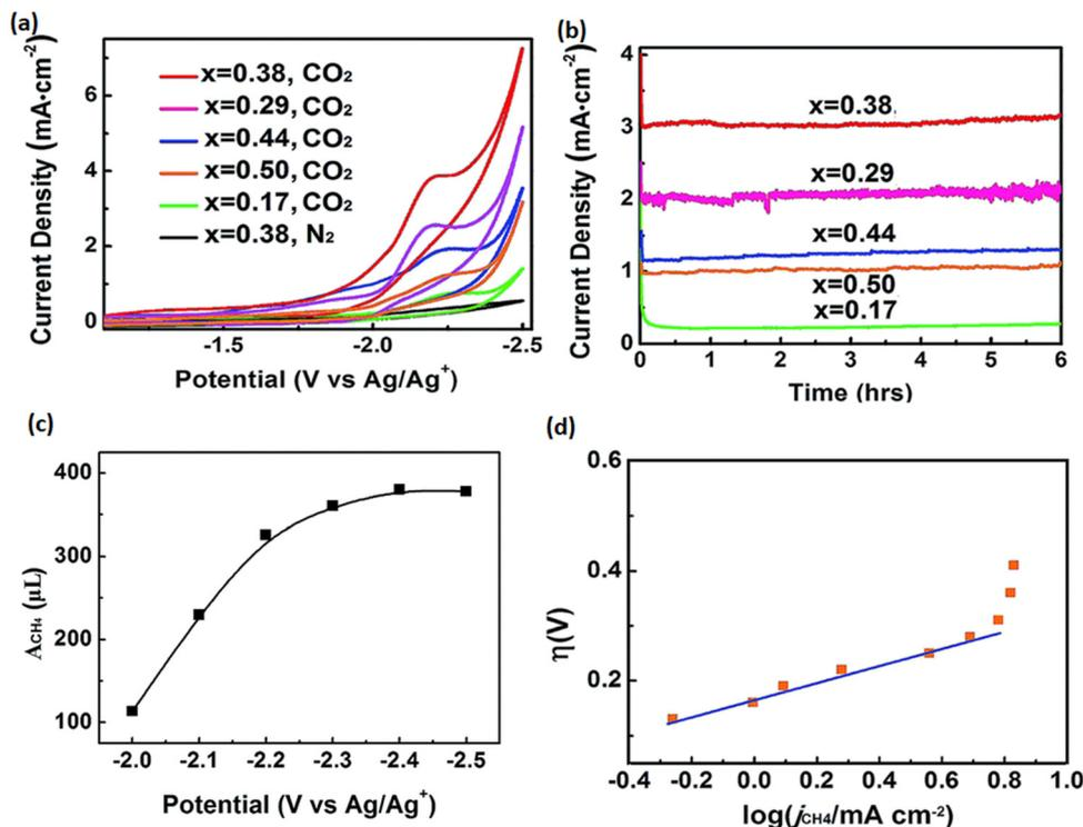
Fig. 15 (a) CV scans in CO<sub>2</sub>-saturated and (b) stability test of different Zn-MOF/CP cathodes. (c) Amount of CH<sub>4</sub> (A<sub>CH<sub>4</sub></sub>, volume at standard temperature and pressure) generated in 2 h under different potentials. (d) Tafel plot for CH<sub>4</sub> of the Zn-MOF/CP cathode using Zn-MOF synthesized at x = 0.38. Reproduced from Kang *et al.*<sup>157</sup> Copyright 2016, Wiley.
