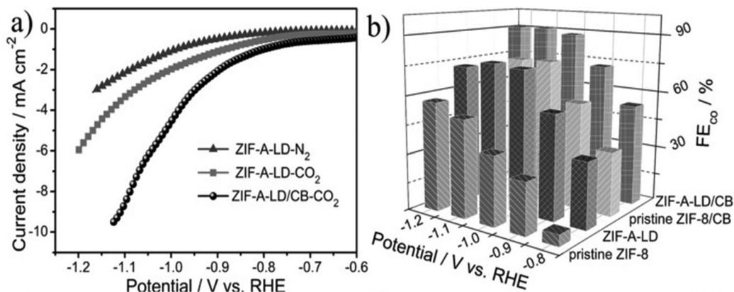
Fig. 16 (a) LSV curves of ZIF-8 activated and 1,10-phenanthroline ligand doped product (ZIF-A-LD) in N<sub>2</sub>- and CO<sub>2</sub>-saturated 0.1 M KHCO<sub>3</sub> solution in comparison with ZIF-A-LD/CB (b) FE<sub>CO</sub>. Reproduced from Dou *et al.*<sup>156</sup> Copyright 2019, Wiley.
