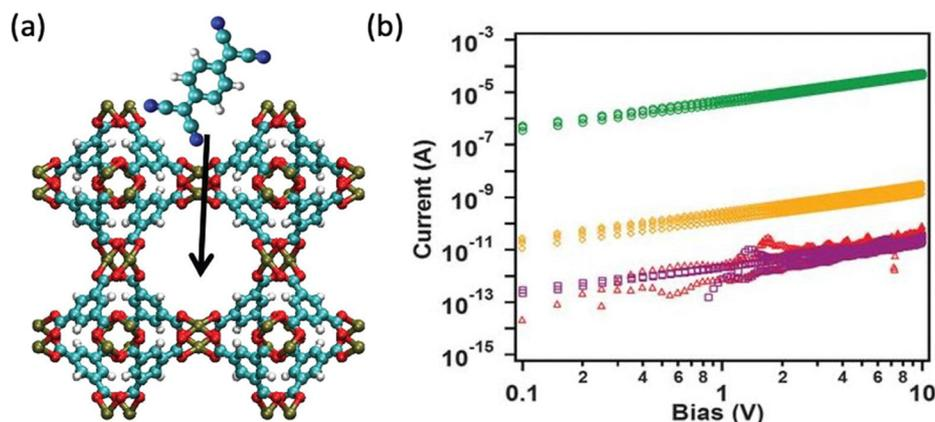
Fig. 2 (a) Fabrication of electrically conductive  $\text{TCNQ}@\text{Cu}_3(\text{BTC})_2$  *via* post-synthetic incorporation (b)  $I$ - $V$  curve showing the electrical conductivity of pristine  $\text{Cu}_3(\text{BTC})_2$  (red), and after infiltration with TCNQ (green), F4-TCNQ (gold) and H4-TCNQ (purple). Reproduced with permission from Talin *et al.*<sup>44</sup> Copyright from The American Association for the Advancement of Science, 2014.
