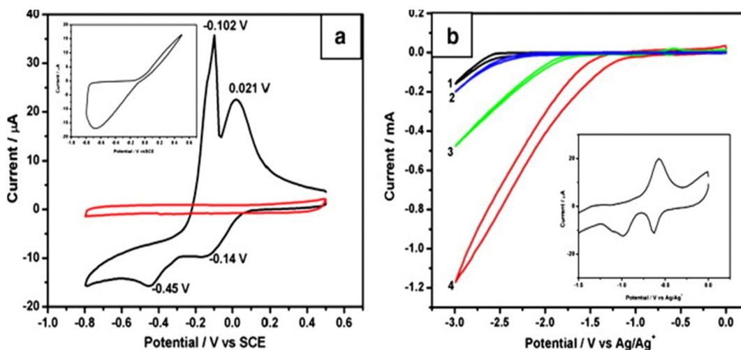
Fig. 12 (a) CV readings of Cu<sub>3</sub>(BTC) + GCE (b) CV scan showing redox activities of (1) GCE, (2) GCE in presence of CO<sub>2</sub>, (3) Cu<sub>3</sub>(BTC)<sub>2</sub> + GCE and (4) Cu<sub>3</sub>(BTC)<sub>2</sub> + GCE in CO<sub>2</sub>-saturated 0.01 M TBATFB/DMF. Reproduced from Kumar *et al.*<sup>112</sup> Copyright 2012, Elsevier.
