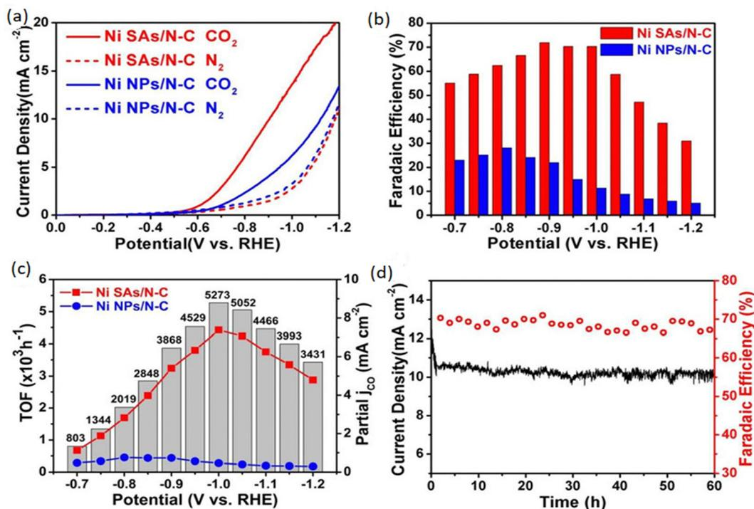
Fig. 20 (a) LSV curves in the  $N_2$ -saturated (dotted line) or  $CO_2$ -saturated (solid line) 0.5 M  $KHCO_3$  electrolyte at a scan rate of  $10\text{ mV s}^{-1}$ . (b) FEs of CO and (c) partial CO current density plots and TOFs of Ni SAs/N-C and Ni NPs/N-C at different applied potentials. (d) Stability of Ni SAs/N-C at a potential of  $-1.0\text{ V vs. RHE}$  for Ni SAs/N-C during 60 h. Reproduced from Zhao et al.<sup>169</sup> Copyright 2017, American Chemistry Society.
