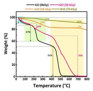
Fig. 8 TGA profiles obtained under nitrogen atmosphere for GO and rGO synthesized at 50 kGy in the absence of silver ions, and rGO-Aq NPs nanocomposites synthesized at 50 kGy (sample A10, series A) and at 70 kGy (sample B10, series B) in presence of silver ions.
