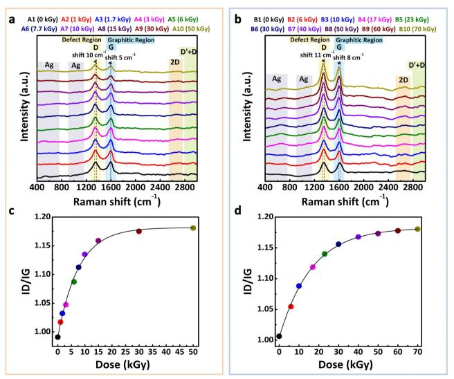
Fig. 6 Raman spectra of non-irradiated and irradiated OG (0.2 g L<sup>-1</sup>)-Ag<sup>+</sup> samples at increasing absorbed doses, taken with a 1 mW laser: (a) series A, (b) series B. Exponential fitting of the  $I_D/I_G$  ratio as a function of the absorbed dose: (c) series A, (d) series B. The uncertainty associated with the obtained values is less than 5%
