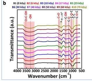
Fig. 5 ATR-FTIR spectra of non-irradiated and irradiated OG (0.2 g L<sup>-1</sup>)-Ag<sup>+</sup> at increasing absorbed doses (under N<sub>2</sub>): (a) [Ag<sup>+</sup>] =  $10^{-3}$  mol L<sup>-1</sup> (series A) and (b)  $[Ag^+] = 10^{-2} \text{ mol } L^{-1} \text{ (series B)}.$
