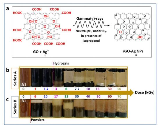
Fig. 1 Schematic representation of the radiolytic synthesis of rGO-Aq NPs in aqueous solution (a). Photographs showing the effect of increasing absorbed dose on the one-step reduction of a degassed aqueous solution containing 0.2 mol  $L^{-1}$  IPA and 0.2 g  $L^{-1}$  of GO together with [Ag<sup>+</sup>]<sub>0</sub> =  $10^{-3}$  mol L<sup>-1</sup> (series A) (b) or [Ag<sup>+</sup>]<sub>0</sub> =  $10^{-2}$  mol L<sup>-1</sup> (series B) (c).
