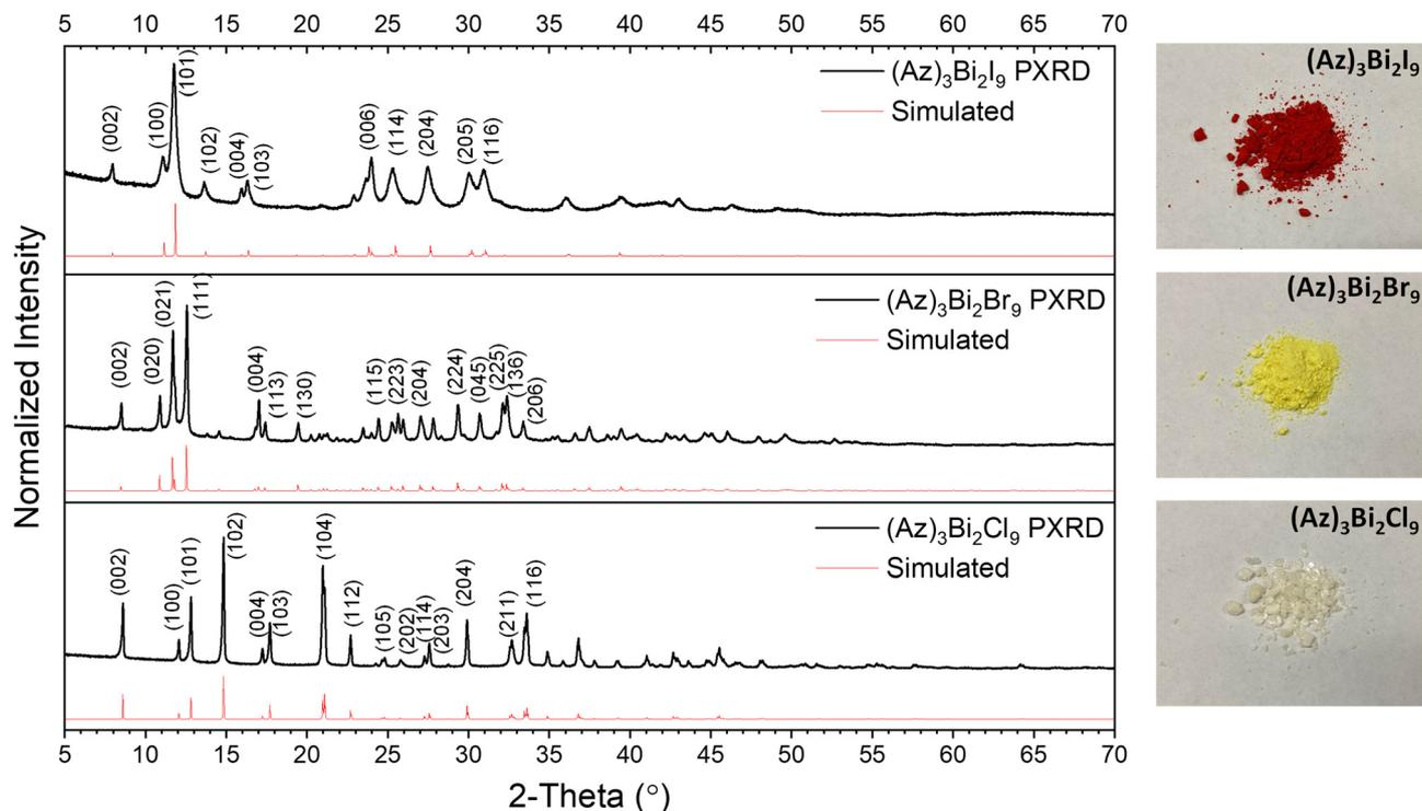
Fig. 3 Powder X-ray diffraction patterns (PXRD) of  $(\text{Az})_3\text{Bi}_2\text{X}_9$  phases with approximately randomly oriented crystals and photographs of the powdered materials. Simulated patterns based on the refined structures are shown for comparison.
