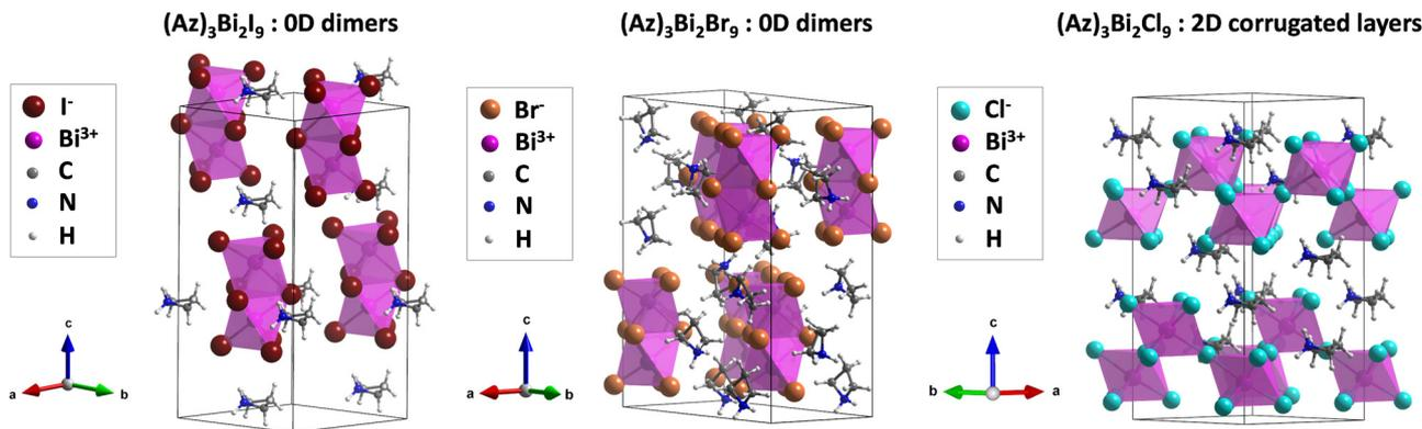
Fig. 2 Refined crystal structure diagrams of  $(\text{Az})_3\text{Bi}_2\text{X}_9$  ( $\text{X} = \text{I}, \text{Br}, \text{Cl}$ ). The azetidinium cations have specific sites in the crystal lattice of  $(\text{Az})_3\text{Bi}_2\text{X}_9$  but a random orientation of the ring. The orientations of the azetidinium ring do not coincide with Rietveld refinement results but represent a snapshot of the disordered cation. (Edited by VESTA software.)
