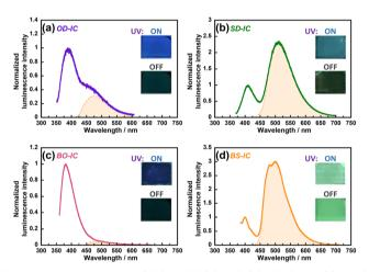
Fig. 5 Emission spectra for (a) OD-IC, (b) SD-IC, (c) BO-IC, and (d) BS-IC dispersed in PMMA films under vacuum. The  $\lambda_{ex}$ s are summarised in Table 1. The areas hatched in orange indicate PH spectral components. Insets are photos of the films under vacuum (UV ON) and just after ceasing UV irradiation (UV OFF).
