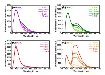
Fig. 6 Irradiation time dependence of the emission spectra of ICs dispersed in PMMA films in air. (a) OD-IC, (b) SD-IC, (c) BO-IC, and (d) BS-IC. The irradiation wavelengths ( $\lambda_{ir}$ ) were set to 340 nm for OD-IC and BO-IC and 365 nm for SD-IC and BS-IC.
