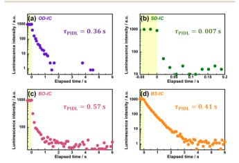
Fig. 8 PIDL decay curves of ICs dispersed in PMMA films for (a) OD-IC  $(\lambda_{\rm ir}, \lambda_{\rm em} = 340, 480 \text{ nm})$ , (b) SD-IC (365, 500 nm), (c) BO-IC (340, 470 nm), and (d) BS-IC (365, 480 nm). The irradiation period is presented by yellow
