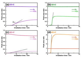
Fig. 7 Time evolution of the emission peak areas during UV irradiation in air for (a) OD-IC, (b) SD-IC, (c) BO-IC, and (d) BS-IC dispersed in PMMA films. The  $\lambda_{ir}$ s of OD-IC and BO-IC was 340 nm and that of SD-IC and BS-IC was 365 nm. The slopes at the onset of PIDL ( $S_{on}$ ) are shown as a
