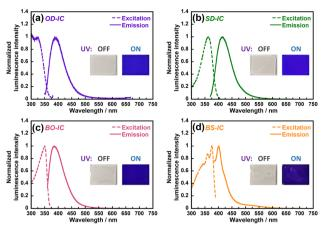
Fig. 4 Excitation/emission spectra for (a) OD-IC, (b) SD-IC, (c) BO-IC, and (d) BS-IC dispersed in PMMA films in air. The excitation wavelength ( $\lambda_{ex}$ ) for the emission spectra and the monitoring emission wavelength ( $\lambda_{em}$ ) for the excitation spectra are summarised in Table 1. Insets are photos of the films under irradiation of white light (UV OFF) and UV light ( $\lambda$  = 365 nm) (UV ON).
