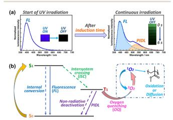
Fig. 1 (a) Variation of emission spectra with continuous UV irradiation and (b) Jablonski diagram based on the photophysical mechanism of PIDL.<sup>26</sup> During the first few minutes of irradiation, ICs exhibit only FL because PH is quenched via OQ. After the continuous irradiation, the OQ efficiency decreases, resulting in the emergence of green PIDL
