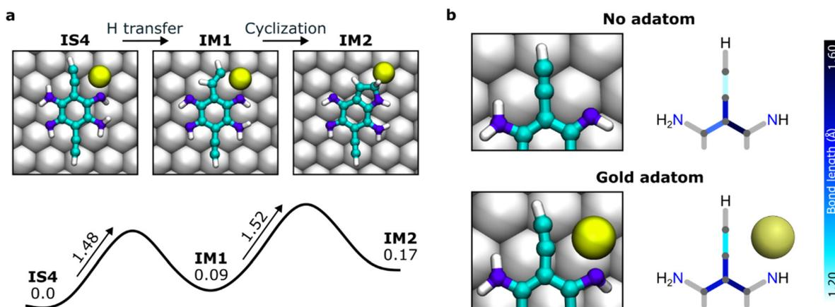
Fig. 2 Reaction pathway of the first hydroamination/cyclization. (a) Simulated snapshots and activation energies of the reaction steps from the initial state **1** (**IS4**), intermediate state 1 (**IM1**) and intermediate state 2 (**IM2**) of the ring closure. (b) Bond length analysis comparison for the effect of gold adatom in the hydrogen transfer step. The model shows an increment of the alkyne length with the presence of a gold adatom leading to a change in the character of the bond.
