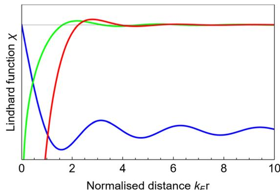
**Fig. 16** Schematic plot of 1D (blue), 2D (green) and 3D (red) Lindhard response functions from Table 1. One can notice the decay being the slowest for the 1D case whereas the fastest for the 3D case.
