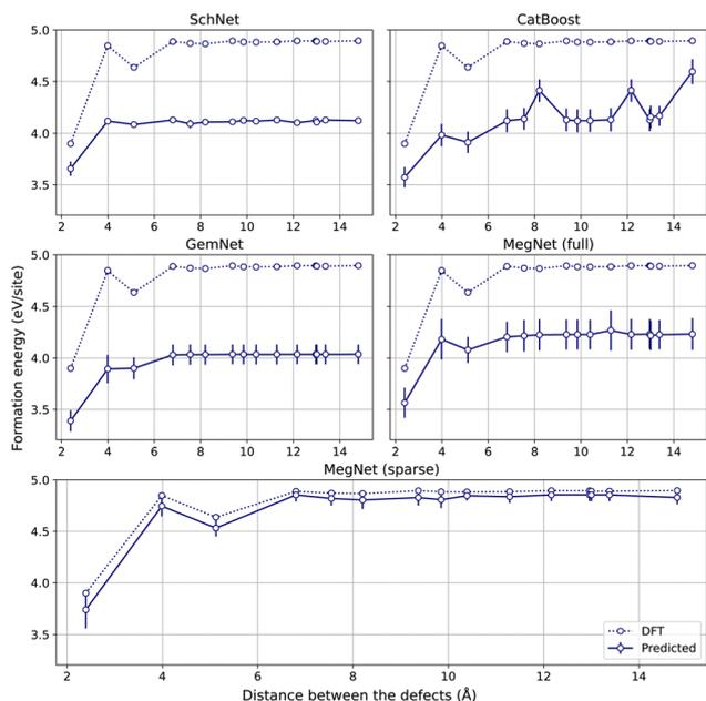
Fig. 31 The dependency of formation energies on the distance between defects in MoS<sub>2</sub> with one Mo and one S vacancy obtained with neural network approaches (SchNet, CatBoost, GemNet, MegNet) and DFT. Reprinted with permission from the work of Kazeev *et al.*<sup>155</sup>
