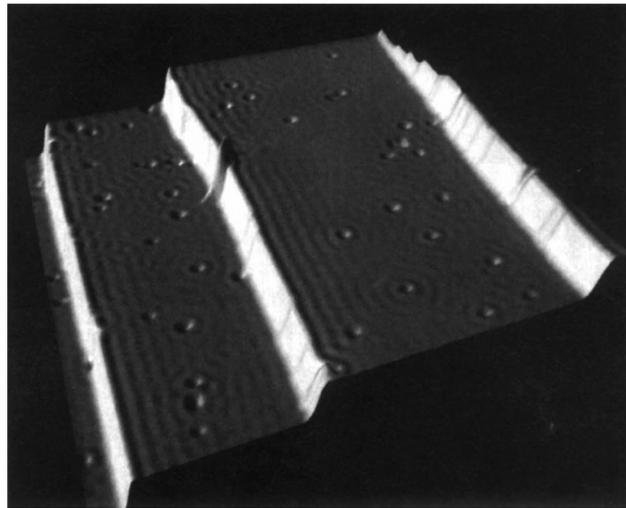
**Fig. 3** Constant-current STM image of the Cu(111) surface. Friedel oscillations from point defects and step edges are clearly visible.<sup>2</sup> Friedel oscillations can be identified by their long-range wave-like pattern. Reprinted with permission from Crommie *et al.*<sup>2</sup>
