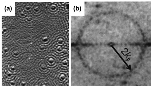
Fig. 7 (a) STM image of the Cu(111) surface obtained at  $-5$  mV bias voltage. (b) Fourier transform of the STM picture (a), showing the ring radius being  $2k_F$ . Please note that the atoms seem to share local density of states oscillations. Panels (a) and (b) are reprinted with permission from the work of Petersen *et al.*<sup>50</sup>
