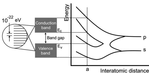
Fig. 5 Scheme showing the dependence of the bandgap on the distance between atoms. It is highly connected to the definition of electron gas.<sup>16</sup> The attempt to classify the electron gas density depends on the distance between AOs or overlapping electronic levels in crystals. One should note here that a chain of atoms can be considered as a 1D crystal and graphene as a 2D crystal.
