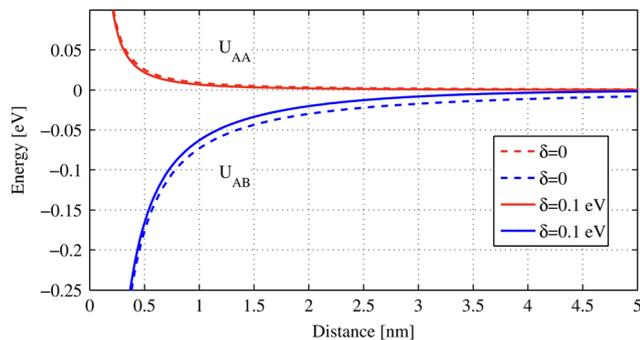
**Fig. 21** Plot of the repulsive (61) and attractive (62) parts of the adatom–adatom indirect interaction through graphene vs. distance. Energy  $\delta$  is associated with the adatom resonance. Reprinted with permission from the work of Shytov *et al.*<sup>132</sup>
