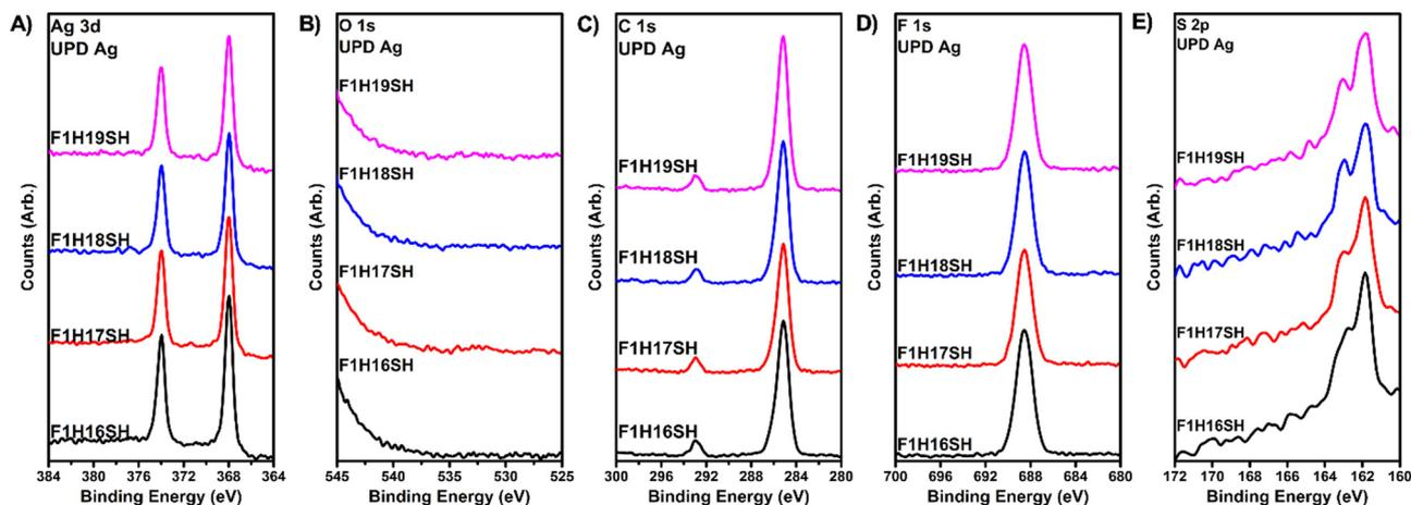
Fig. 6 XPS spectra for the (A) Ag 3d, (B) O 1s, (C) C 1s, (D) F 1s, and (E) S 2p region for the **F1HmSH** SAMs on UPD Ag.
