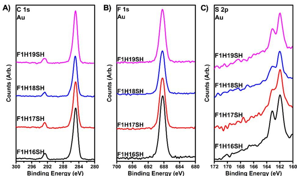
Fig. 5 XPS spectra for the (A) C 1s, (B) F 1s, and (C) S 2p region for the **F1H<sub>m</sub>SH** SAMs on Au.
