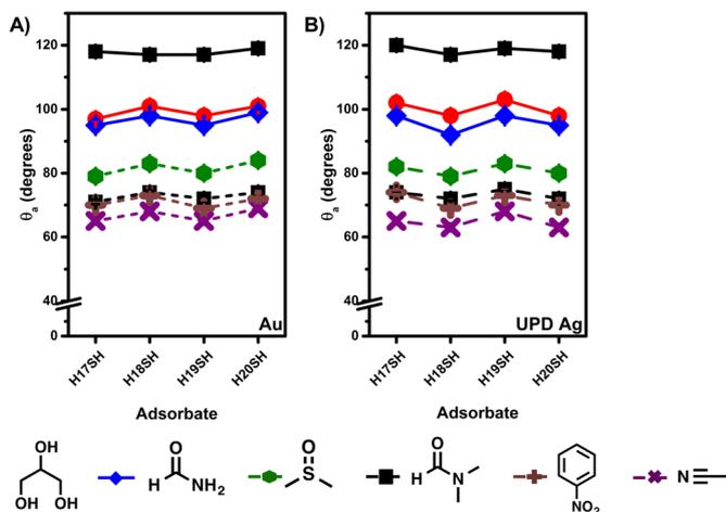
Fig. 11 Advancing contact angles for H<sub>2</sub>O, GL, FA, DMSO, DMF, NB, and ACN on  $H_nSH$  SAMs on (A) Au and (B) UPD surfaces. Error bars fall within the symbols.
