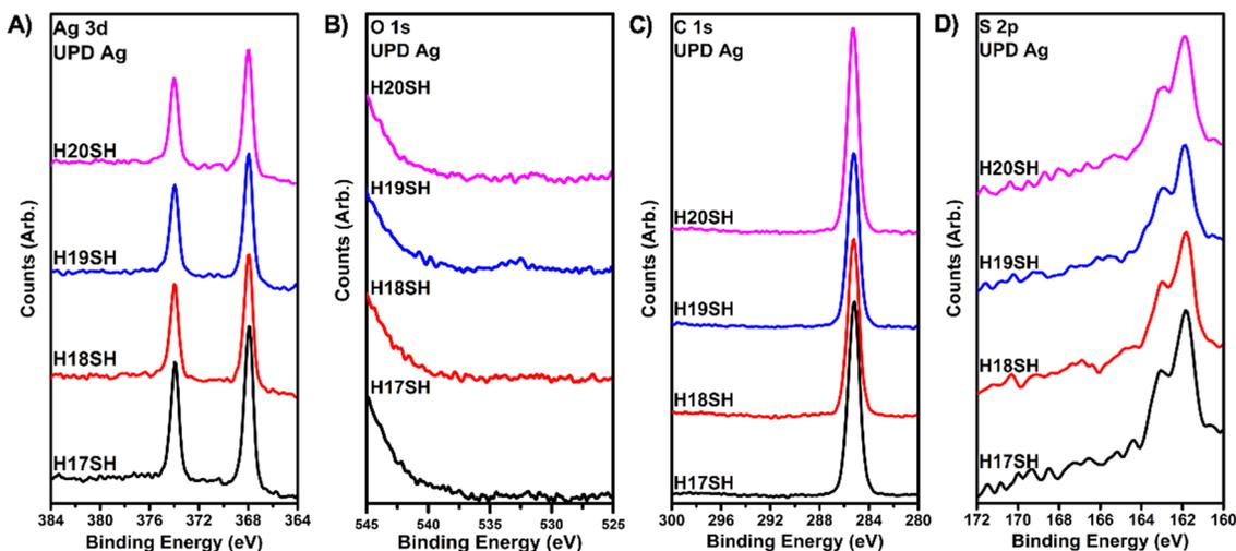
Fig. 4 XPS spectra for the (A) Ag 3d, (B) O 1s, (C) C 1s, and (D) S 2p region for the **H<sub>n</sub>SH** SAMs on UPD Ag.
