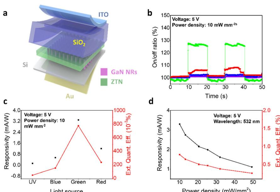
**Fig. 5** (a) Schematic illustration of the DH-PD with the ZNT/GaN NRs/Si structure. (b) Operation properties of DH-PD. (c) The results of light-selectivity of the DH-PD. (d) The performance test results of the DH-PD.
