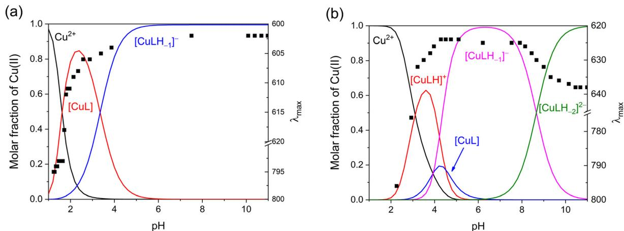
**Fig. 1** Distribution of the complexes formed in the Cu(II)–PyHis (a) and Cu(II)–PydiHis (b) systems at a 1:1 metal ion to ligand ratio and the  $\lambda_{\max}$  value of the d–d band (■) obtained by UV-vis spectroscopy as a function of pH.  $c_{\text{Cu(II)}} = 1.81 \text{ mM}$ ,  $c_{\text{PyHis}} = 1.90 \text{ mM}$  and  $c_{\text{PydiHis}} = 1.90 \text{ mM}$ .
