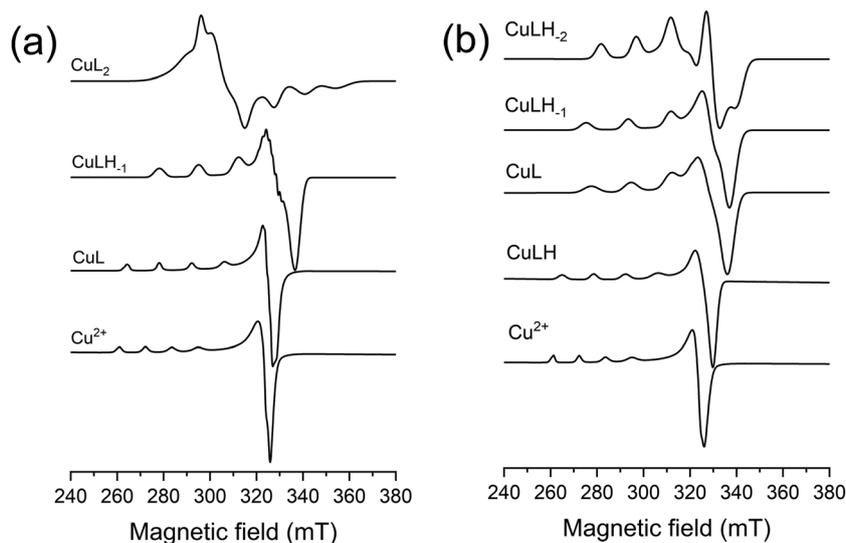
**Fig. 3** Calculated component EPR spectra obtained for the Cu(II)–PyHis (a) and Cu(II)–PydiHis (b) complexes based on evaluation of the pH-dependent CW-EPR spectra of the frozen solution (see the SI for simulation of the experimental spectra).
