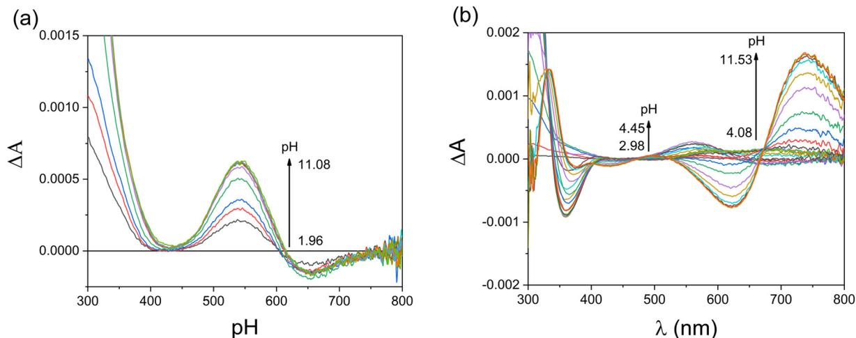
**Fig. 2** CD spectra of the Cu(II) : PyHis (a) and PydiHis (b) systems at a 1:1 metal ion to ligand concentration ratio as a function of pH.  $c_{\text{Cu(II)}} = 0.95 \text{ mM}$ .
