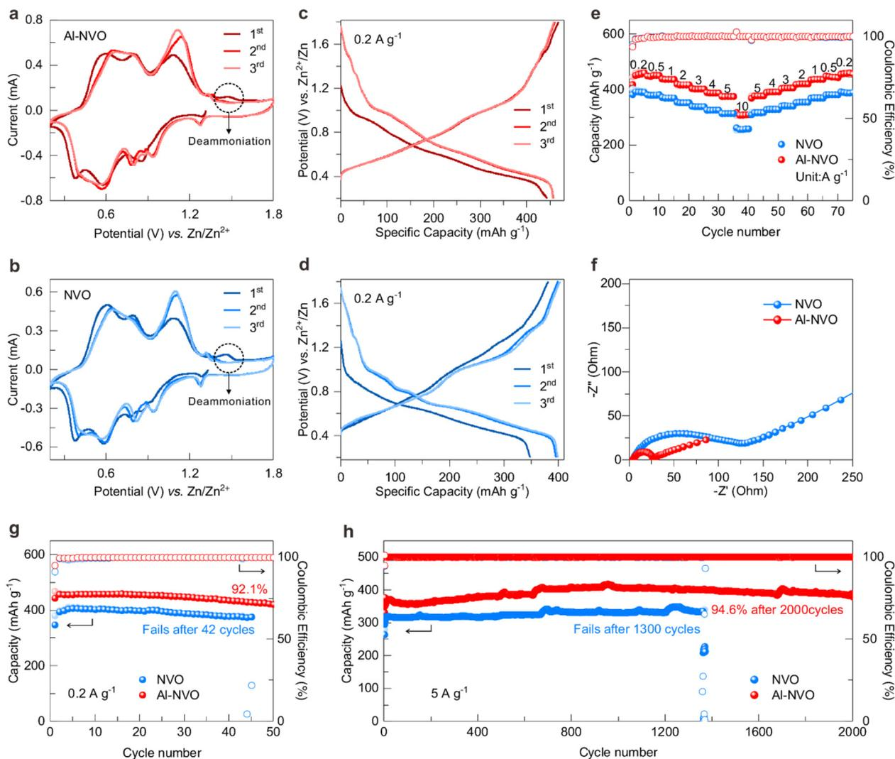
**Fig. 2** Electrochemical characterization of Al-NVO and NVO cathodes. (a and b) CV profiles during the initial three cycles. (c and d) GCD curves at  $0.2 \text{ A g}^{-1}$ . (e) Rate performance across current densities ( $0.2\text{--}10 \text{ A g}^{-1}$ ). (f) Nyquist plots. Cycling stability at (g)  $0.2$  and (h)  $5 \text{ A g}^{-1}$ , respectively.
