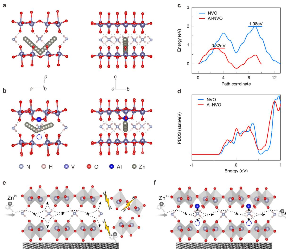
**Fig. 4** DFT calculations: theoretical migration pathways for  $\text{Zn}^{2+}$  in (a) NVO and (b) Al-NVO. (c) Calculated  $\text{Zn}^{2+}$  diffusion barriers in NVO and Al-NVO cathodes. (d) DOS analysis for NVO and Al-NVO cathodes. Schematic diagrams comparing structural stability evolution of (e) NVO and (f) Al-NVO cathodes during electrochemical cycling.
