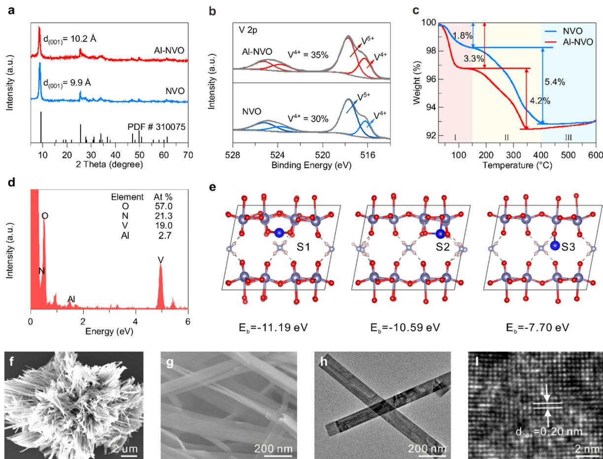
**Fig. 1** Phase and structural analyses of Al-NVO and NVO (a) XRD patterns. (b) V 2p XPS spectra. (c) TG profiles under air atmosphere. (d) EDS of the Al-NVO. (e) Computational models and corresponding adsorption energies of Al atoms at three distinct lattice sites (S1–S3). (f and g) SEM, (h) TEM and (i) HR-TEM images of Al-NVO.
