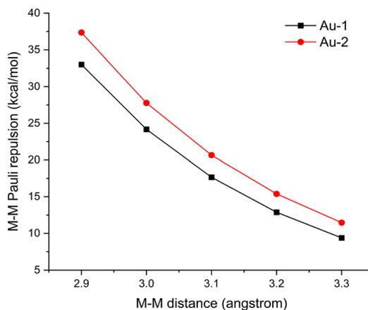
**Fig. 9** Calculated M–M Pauli repulsion of **Au-1** and **Au-2** dimers by changing the M–M distance. For EDA calculations at non-equilibrium M–M distances, fragment geometries were frozen while varying metal–metal separation.
