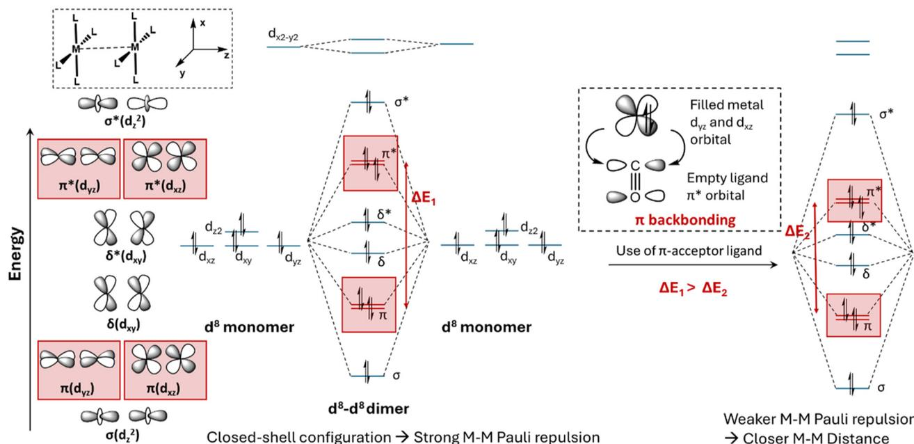
**Scheme 2** Schematic illustration of the role of the  $\pi$ -acceptor ligand in weakening the M–M Pauli repulsion for  $d^8$ – $d^8$  closed-shell metal complexes. Schematic illustration of the MO for  $d^{10}$ – $d^{10}$  closed-shell metal complexes has been provided in the ESI.†
