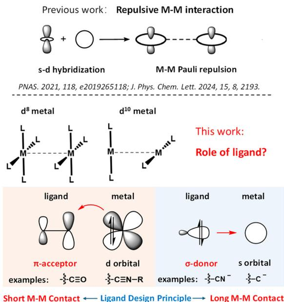
**Scheme 1** Top: previous work, repulsive M–M interaction in closed-shell d<sup>8</sup> and d<sup>10</sup> transition metal complexes. Bottom: this work, the role of π-acceptor and σ-donor ligands in M–M interactions.
