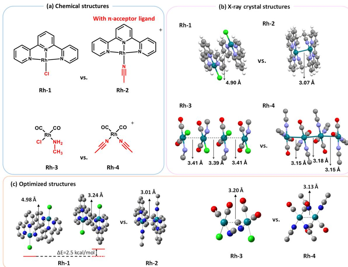
**Fig. 1** Chemical structures (a), X-ray crystal structures (b) and optimized structures (c) of  $d^8$  Rh(I) metal complexes with or without  $\pi$ -acceptor ligands studied in this work. Calculations were performed at the PBE0-GD3BJ/SDD(Rh)/6-31G\* (other elements) level of theory using the PCM solvent model for acetonitrile (ACN) in Gaussian 16.
