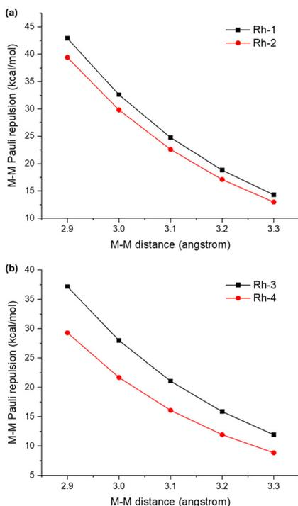
**Fig. 4** Calculated M–M Pauli repulsion of (a) **Rh-1** and **Rh-2** dimers and (b) **Rh-3** and **Rh-4** dimers, by changing the M–M distance. For EDA calculations at non-equilibrium M–M distances, fragment geometries were frozen while varying metal–metal separation.
