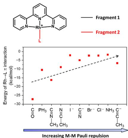
**Fig. 6** Calculated EDA-NOCV deformation orbital energies correspond to the  $\text{Rh} \rightarrow \text{L} \pi$  interaction in the model system of  $\text{Rh}(\text{terpy})\text{L}$ . All data points are tabulated in Table S1.†
