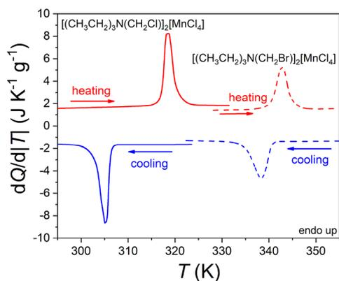
**Fig. 1** VT-DSC curves at ambient pressures for  $[(\text{CH}_3\text{CH}_2)_3\text{N}(\text{CH}_2\text{Cl})]_2[\text{MnCl}_4]$  (solid lines) and  $[(\text{CH}_3\text{CH}_2)_3\text{N}(\text{CH}_2\text{Br})]_2[\text{MnCl}_4]$  (dash lines) from 295 to 355 K.
