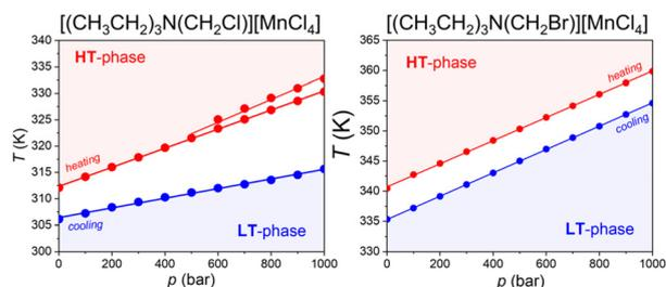
**Fig. 7**  $p$  $T$  phase diagram of  $[(\text{CH}_3\text{CH}_2)_3\text{N}(\text{CH}_2\text{Cl})]_2[\text{MnCl}_4]$  (left) and  $[(\text{CH}_3\text{CH}_2)_3\text{N}(\text{CH}_2\text{Br})]_2[\text{MnCl}_4]$  (right) from 1 bar to 1000 bar.
