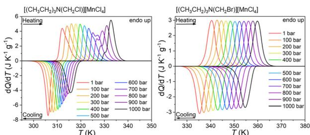
**Fig. 6** VT-DSC curves of  $[(\text{CH}_3\text{CH}_2)_3\text{N}(\text{CH}_2\text{Cl})]_2[\text{MnCl}_4]$  (left) and  $[(\text{CH}_3\text{CH}_2)_3\text{N}(\text{CH}_2\text{Br})]_2[\text{MnCl}_4]$  (right) under isobaric conditions from 1 bar to 1000 bar.
