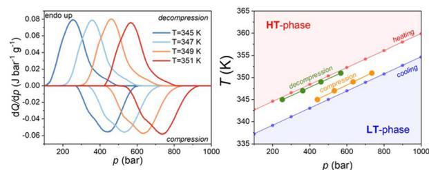
**Fig. 9** (Left) VP-DSC curves of  $[(\text{CH}_3\text{CH}_2)_3\text{N}(\text{CH}_2\text{Br})]_2[\text{MnCl}_4]$  under isothermal conditions from 345 to 351 K. (Right)  $pVT$  phase diagram of  $[(\text{CH}_3\text{CH}_2)_3\text{N}(\text{CH}_2\text{Br})]_2[\text{MnCl}_4]$  comparing data obtained from isothermal and isobaric DSC measurements.
