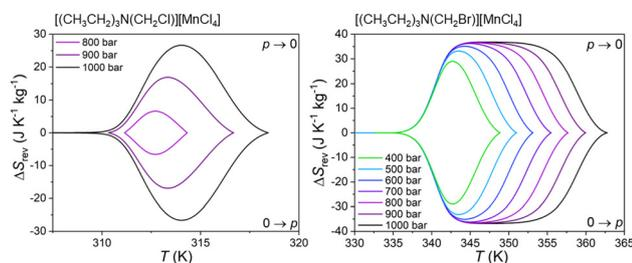
**Fig. 8** Reversible isothermal entropy changes on applying ( $0 \rightarrow p$ ) and removing ( $p \rightarrow 0$ ) pressure obtained by quasidirect methods of  $[(\text{CH}_3\text{CH}_2)_3\text{N}(\text{CH}_2\text{Cl})]_2[\text{MnCl}_4]$  (left) and  $[(\text{CH}_3\text{CH}_2)_3\text{N}(\text{CH}_2\text{Br})]_2[\text{MnCl}_4]$  (right).
