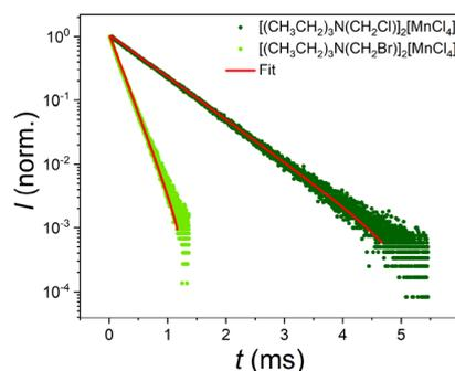
**Fig. 14** Emission decay curves for  $[(\text{CH}_3\text{CH}_2)_3\text{N}(\text{CH}_2\text{Cl})_2][\text{MnCl}_4]$  and  $[(\text{CH}_3\text{CH}_2)_3\text{N}(\text{CH}_2\text{Br})_2][\text{MnCl}_4]$  compounds at room temperature.
