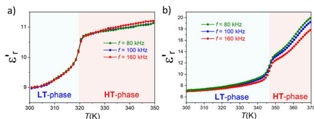
**Fig. 10** Temperature-dependence of the dielectric permittivity of  $[(\text{CH}_3\text{CH}_2)_3\text{N}(\text{CH}_2\text{X})]_2[\text{MnCl}_4]$  where (a)  $X = \text{Cl}$  and (b)  $X = \text{Br}$  during the heating and cooling runs, at 80, 100 and 160 kHz.
