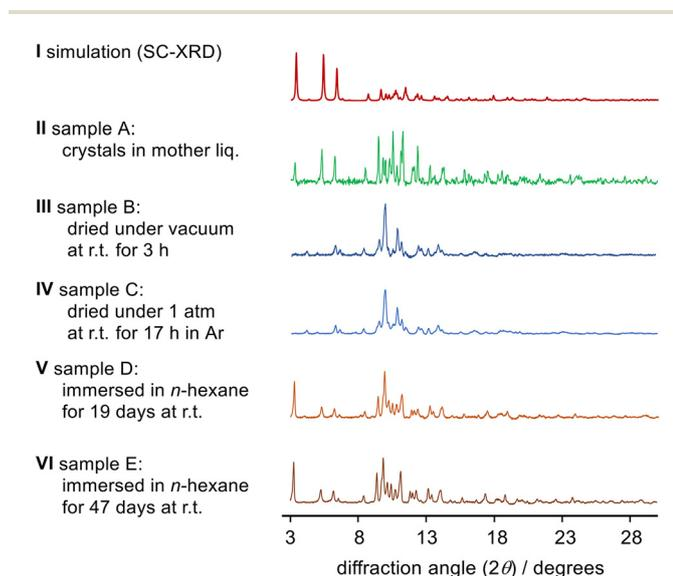
**Fig. 4** Powder X-ray diffraction patterns of **4**. I: the simulation pattern obtained from the SC-XRD analysis; II: the PXRD pattern of sample A – crystals in mother liq.; III: sample B – dried under vacuum; IV: sample C – dried under Ar; V: sample D – immersed in *n*-hexane for 19 days at r. t.; and VI: sample E – immersed in *n*-hexane for 47 days at r. t. ( $2\theta = 3\text{--}30^\circ$ ).
