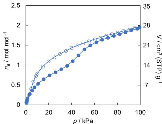
**Fig. 5** Adsorption isotherm of CO<sub>2</sub> at 195 K. The solid and open circles in blue represent adsorption and desorption, respectively.
