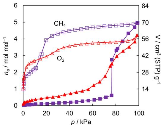
**Fig. 6** Adsorption isotherms of CH<sub>4</sub> (112 K) and O<sub>2</sub> (90 K). The solid-open square and triangle represent the adsorption–desorption of CH<sub>4</sub> and O<sub>2</sub>, respectively.
