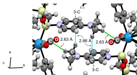
**Fig. 3** CH– $\pi$  interaction in the crystal of **4** around the dmap ligands: atomic codes W, light blue; C, grey; N, purple; O, red; Si, light yellow; and H, white. Blue line: CH– $\pi(\text{py})$ , green line: CH– $\pi(\text{CO})$  interaction.
