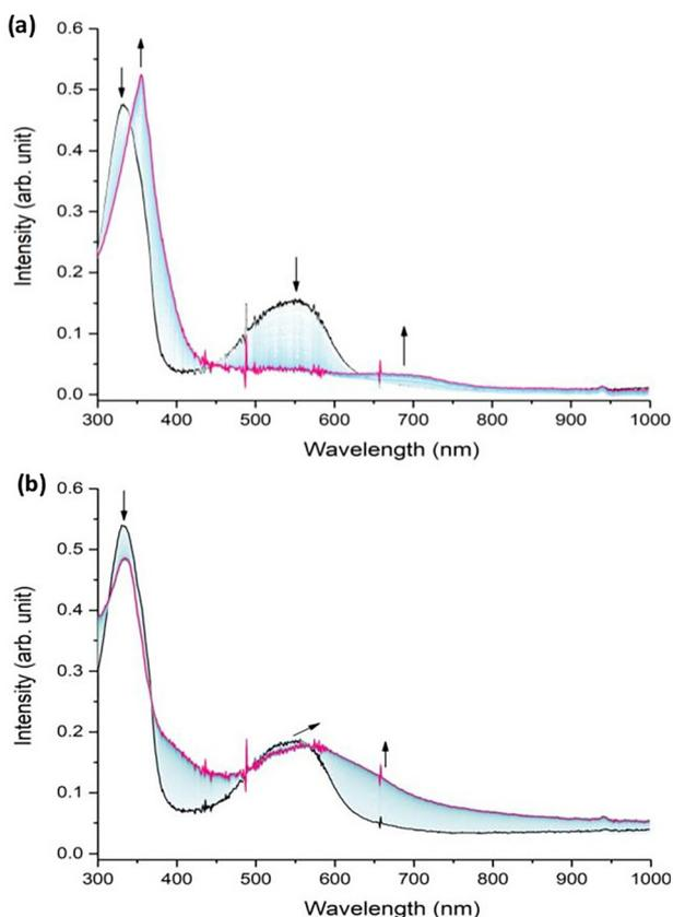
**Fig. 3** *In situ* UV-VIS spectra of *fac*-C2 (0.2 mM) in an acetonitrile solution containing 0.1 M TBAPF<sub>6</sub>. (a) during exhaustive oxidation at  $E_{\text{app}} = 1.2$  V vs. SCE (last scan after 285 s), (b) during exhaustive reduction at  $E_{\text{app}} = -1$  V vs. SCE (last scan after 570 s) (pathlength of 1 mm and scan delay of 5 s between two spectra).
