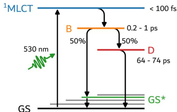
Fig. 8 Proposed relaxation scheme for the family of complexes. The <sup>1</sup>MLCT is populated and depleted within less than 100 fs. Its depopulation corresponds to the population of state **B** that decays over the ps timescale into a hot ground state **GS\*** and the long-living state **D**.
