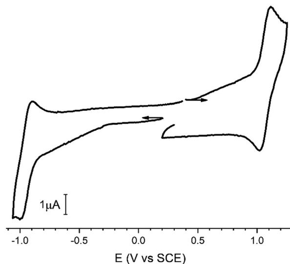
**Fig. 2** Cyclic voltammogram of *fac*-C2 (0.2 mM) in a MeCN solution containing 0.1 M TBAPF<sub>6</sub>, recorded at  $\nu = 100$  mV s<sup>-1</sup>.
