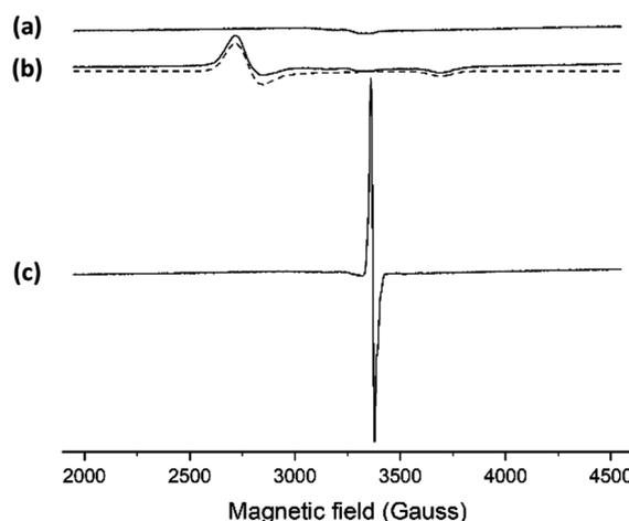
**Fig. 4** X-band cw-EPR spectra recorded at 100 K of a MeCN solution of *fac*-C2 (0.2 mM) containing 0.1 M TBAPF<sub>6</sub>. (a) Initial Fe(II) complex, (b) after exhaustive electrolysis at  $E_{\text{app}} = 1.2$  V vs. SCE. Simulation in dashed line for a low-spin  $S = 1/2$  Fe(III) complex with  $g_{\perp} = 2.452$  and  $g_{\parallel} = 1.823$ , (c) after exhaustive electrolysis at  $E_{\text{app}} = -1$  V vs. SCE to generate an Fe(II)L<sup>•−</sup> radical with  $g = 1.999$ .
