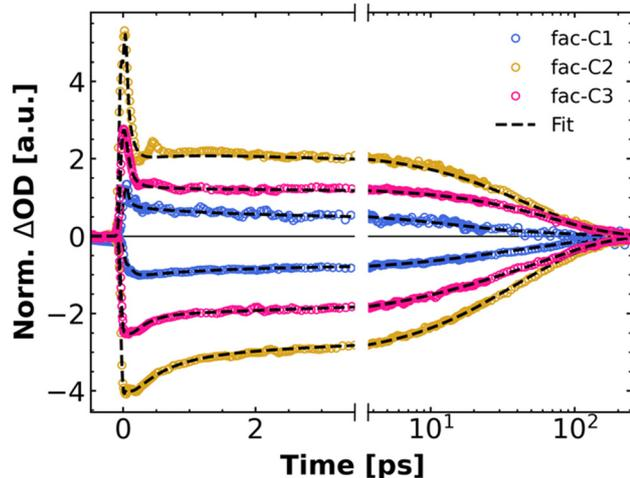
Fig. 7 Comparison of temporal decay traces of complexes *fac-C1* (blue), *fac-C2* (orange), and *fac-C3* (pink). Best fits are represented by black dashed lines. Kinetics were chosen at a maximum of ESA and GSB for all complexes, respectively at 370 nm, 380 nm, and 335 nm (ESA) and 555 nm, 555 nm, and 500 nm (GSB). For the sake of clarity, kinetics were normalised and separated by the application of a scaling factor.
