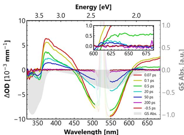
**Fig. 5** Selected differential transient absorption spectra of complex *fac*-C2. Excitation wavelength 530 nm. The sign-inverted and arbitrarily scaled ground state absorption is plotted for comparison (grey). Inset: zoom into the 600–700 nm region highlighting the narrowing of the red ESA between 0.5 and 20 ps delay.
