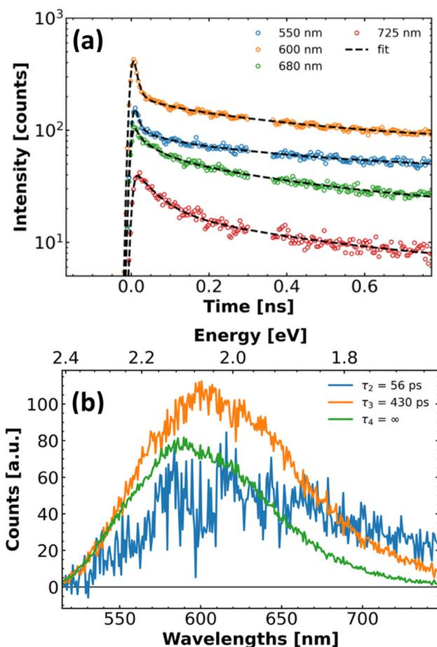
**Fig. 10** Time-resolved emission data of *fac*-C2 recorded with a streak camera (10 ps time resolution FWHM). Excitation with 0.3 ps pulses at 515 nm, and detection through a long-pass OG550 filter. (a) Kinetic traces of the time-dependent luminescence measurement with best fits as dashed lines. (b) Decay-associated spectra (DAS) of the different lifetimes found by global analysis.
