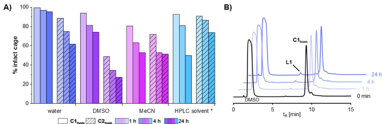
Fig. 4 (A) Stability study of **C1<sub>hom</sub>** and **C2<sub>hom</sub>** in different solvents analysed by RP-HPLC. The theoretical cage concentration after dilution with the respective solvent was 0.1 mM. \*MeCN/ $\text{H}_2\text{O}$  (1/1) +0.1% TFA. (B) Stability of **C1<sub>hom</sub>** in Milli-Q  $\text{H}_2\text{O}$  monitored over 24 h by RP-HPLC (40–70% B in 15 min).
