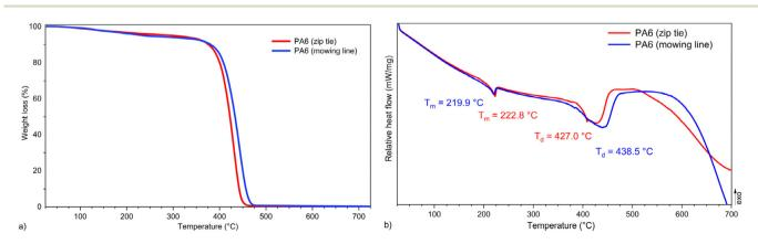
Fig. 10 TGA (a) and DSC (b) thermograms of PA6 zip ties and mowing lines investigated in alcoholysis reactions.
