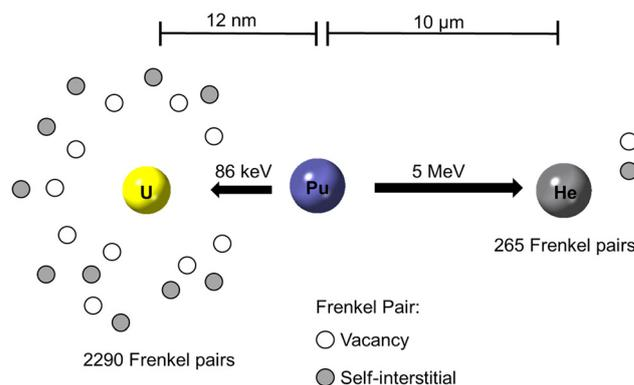
Fig. 12 Representation of Frenkel defect formation in  $\delta$ -Pu. Adapted from Wolfer.<sup>212</sup>
