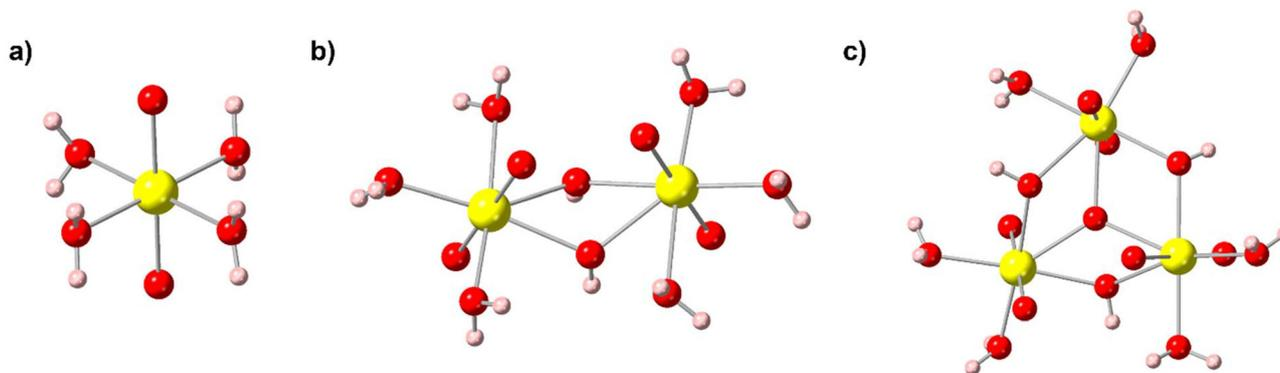
**Fig. 7** Uranyl ( $\text{UO}_2^{2+}$ ) complexes that can exist in aqueous solutions with hydroxide anions. (a)  $[\text{UO}_2(\text{H}_2\text{O})_4]^{2+}$ , (b)  $[\text{UO}_2(\text{OH})_2(\text{H}_2\text{O})_4]^{2+}$ , and (c)  $[\text{UO}_2(\text{O})(\text{OH})_3(\text{H}_2\text{O})_4]^+$ . U, O, and H are depicted as yellow, red, and pink spheres, respectively. Adapted from Quilès *et al.*<sup>71</sup>
