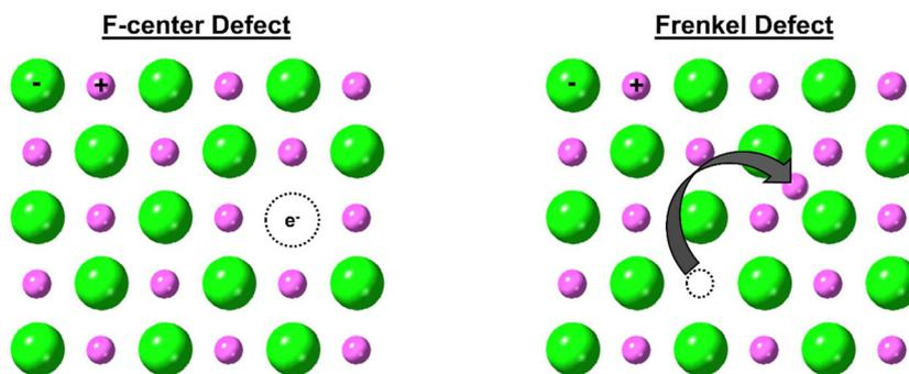
**Fig. 11** Model of F-center defects (left) and Frenkel defects (right) in the solid-state. Cation and anions are represented by pink and green spheres, respectively, whereas the dashed circle represents a vacancy site. Adapted from Leitner *et al.*<sup>202</sup>
