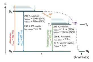
Fig. 5 Jablonski diagram of compound 1 including the intermolecular TTA process with a second molecule of 1 acting as annihilator (ISC = crossing, TTA = triplet-triplet annihilation, PS = intersystem polystyrene).
