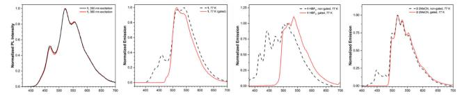
Fig. 6 Emission spectra of a polystyrene film of 1 (1% w/w) at ambient temperature (left) and 10 μM solution of 1, 1·HBF4 and 2·2MeCN recorded in glassy 2-methyl-THF at 77 K. The excitation wavelength was 360 nm. The dashed line contains both fluorescence and phosphorescence, whereas in the gated spectrum (red line) the fluorescence is suppressed. These spectra are independent on concentration.
