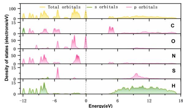
**Fig. 4** The total and partial density of states.
