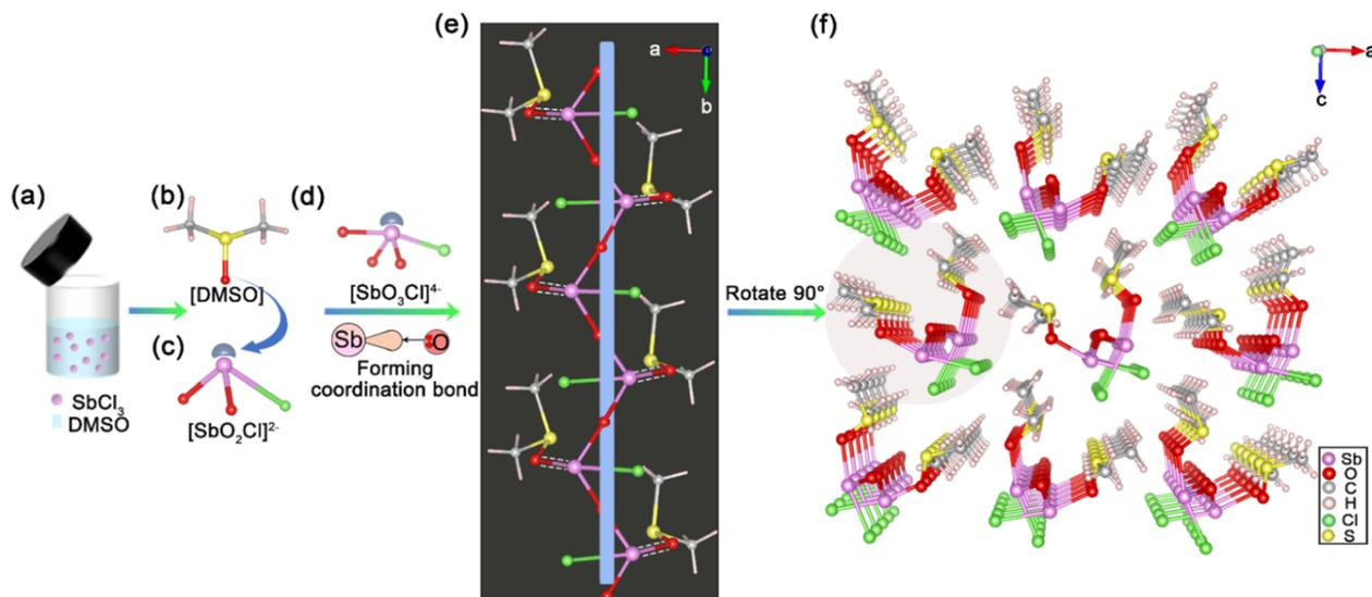
**Fig. 2** (a) Schematic diagram of the synthetic route; ball and stick representations of (b) the [DMSO] and (c)  $[\text{SbO}_2\text{Cl}]^{2-}$  triangular pyramids; (d)  $[\text{SbO}_3\text{Cl}]^{4-}$  seesaw; (e) the 1D  $[\text{SbOClDMSO}]_\infty$  organic–inorganic hybrid spiral chain; (f) the 3D framework structure of  $\text{SbOCl}\cdot\text{DMSO}$  viewed in the  $ac$  plane.
