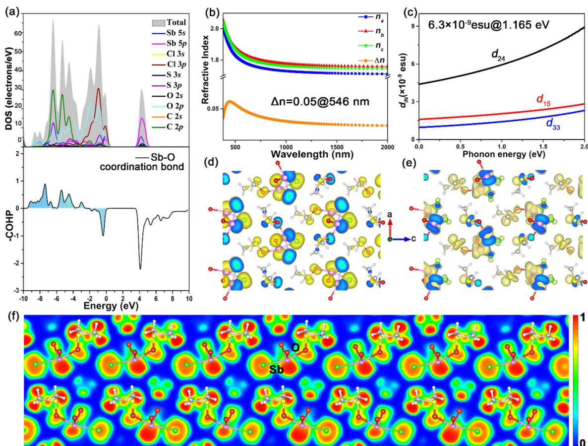
**Fig. 6** (a) The total DOS, partial DOS and –COHP; (b) the calculated linear refractive indices; (c) the calculated frequency-dependent SHG coefficients for SbOCl-DMSO; the SHG density for (d) occupied and (e) unoccupied states in the VE process in SbOCl-DMSO; (f) the ELF map for SbOCl-DMSO.
