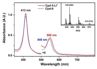
Fig. 2 UV-vis spectra of [Fe<sup>IV</sup>(OLi)(TDFPP)] (red line) and [Fe<sup>IV</sup>(O) (TDFPP)] (blue dashed line) generated through the reaction of [Fe (TDFPP)Cl] (0.05 mM) and PhIO (0.4 mM) in the presence or absence of LiBr in CH<sub>3</sub>CN at 263 K. Inset shows the ESI-MS spectrum of the iron (IV)-oxo species generated in the bromination reaction under standard conditions. m/z = 835.0992:  $[Fe^{V}(OLi)(TDFPP)]^{+}$ ; m/z = 870.0702: [Fe<sup>IV</sup>(OLi)(TDFPP)\*Cl]+.
