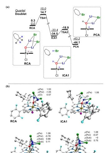
Fig. 3 (a) Gibbs free energy profile (kcal mol<sup>-1</sup>) for the bromination of CHA by Cpd I with two LiBr molecules. (b) Key structures on the doublet involved in the reactions. Key distances (in angstroms) and spin population are given. Some atoms are omitted for clarity.
