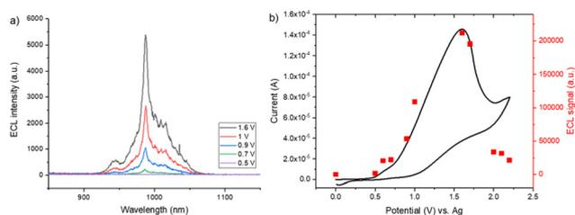
**Fig. 2** (a) Evolution of the ECL spectra of **1Ru–Yb** as a function of the imposed potential. (b) Cyclic voltammogram (black line) and corresponding ECL signal (red squares) recorded in a  $\text{CH}_2\text{Cl}_2$  solution containing 0.5 mM **1Ru–Yb**, 100 mM TPrA and 0.2 M TBAPF<sub>6</sub>. Scan rate: 0.05 V s<sup>-1</sup>. The ECL signals (red squares) have been calculated by recording the ECL spectra at different constant potentials and integrating the emission from 900 nm to 1100 nm.
