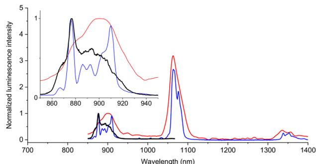
**Fig. 3** Comparison of the normalized ECL (black line) and PL emission spectra of **1Ru-Nd** at room temperature (red line,  $\lambda_{\text{exc}} = 450$  nm) and at 77 K in frozen organic glass (blue line) with the same experimental conditions as in Fig. 2. The ECL spectra of **1Ru-Nd** were recorded at an imposed potential of 1.9 V. The inset shows a zoomed-in view of the 850–950 nm area.
