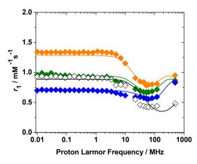
Fig. 8  $^{1}$ H NMRD profiles at 298 K of [Fe(NOTA)] ( $\blacklozenge$ ) (pH = 7.5), [Fe (DETA)] ( $\blacklozenge$ ) (pH = 4.3), [Fe(UNTA)] ( $\blacklozenge$ ) (pH = 7.0) and [Fe(DOTRA)] ( $\diamondsuit$ ) (pH = 7.0).
