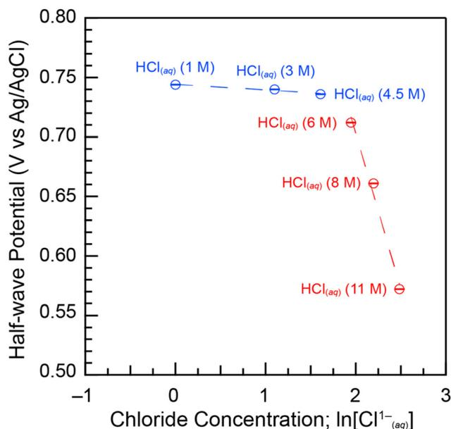
**Fig. 8** Half-wave potentials ( $E_{1/2}$ ) from cyclic voltammetry measurements made on plutonium dissolved in  $\text{HCl}_{(\text{aq})}$  (1–11 M) solutions plotted as a function of the natural log of the  $\text{HCl}_{(\text{aq})}$  concentration. Error bars are the standard deviation of  $E_{1/2}$  measured at eight scan rates from 0.01 to  $10 \text{ V s}^{-1}$ .
