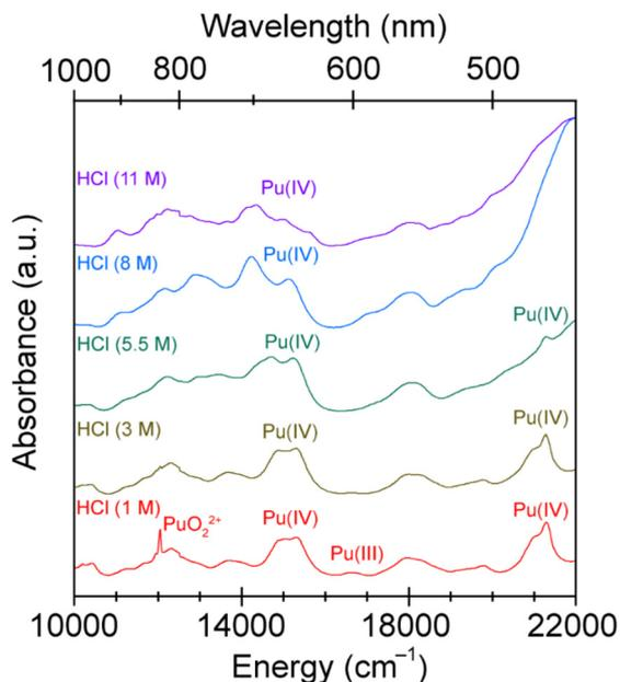
**Fig. 2** Room temperature UV-Vis-NIR spectra from  $\text{Pu}^{4+}_{(\text{aq})}$  after dissolution in  $\text{HCl}_{(\text{aq})}$  solutions (1–11 M from bottom to top) collected immediately after sample preparation. Relevant peaks were labeled with their associated plutonium oxidation states.
