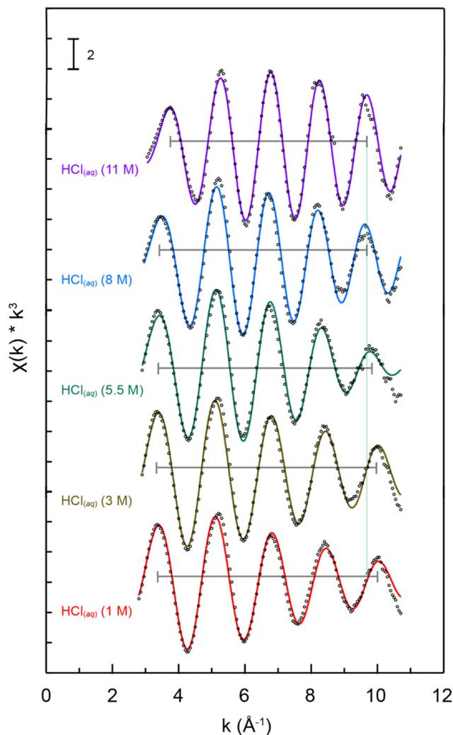
**Fig. 3** The  $k^3$ -weighted room temperature Pu  $L_3$ -edge EXAFS spectra displaying the  $\chi(k)$  function (points) with non-linear curve fitting (lines) from aqueous  $\text{Pu}^{4+}$  solutions in  $\text{HCl}_{(\text{aq})}$  solutions (1–11 M). The gray bracket and the vertical green line were included to help visualize that the wavelength changed with changing  $\text{HCl}_{(\text{aq})}$  concentration.
