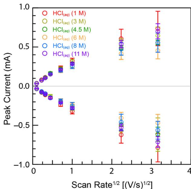
Fig. 6 Peak current (*i*<sub>p</sub>) from cyclic voltammetric measurements made on plutonium (16.7 mM) in HCl<sub>(aq)</sub> (1–11 M) solutions plotted as a function of scan rate (0.01–1 V s<sup>-1</sup>). Error bars are the standard deviation from three replicates.
