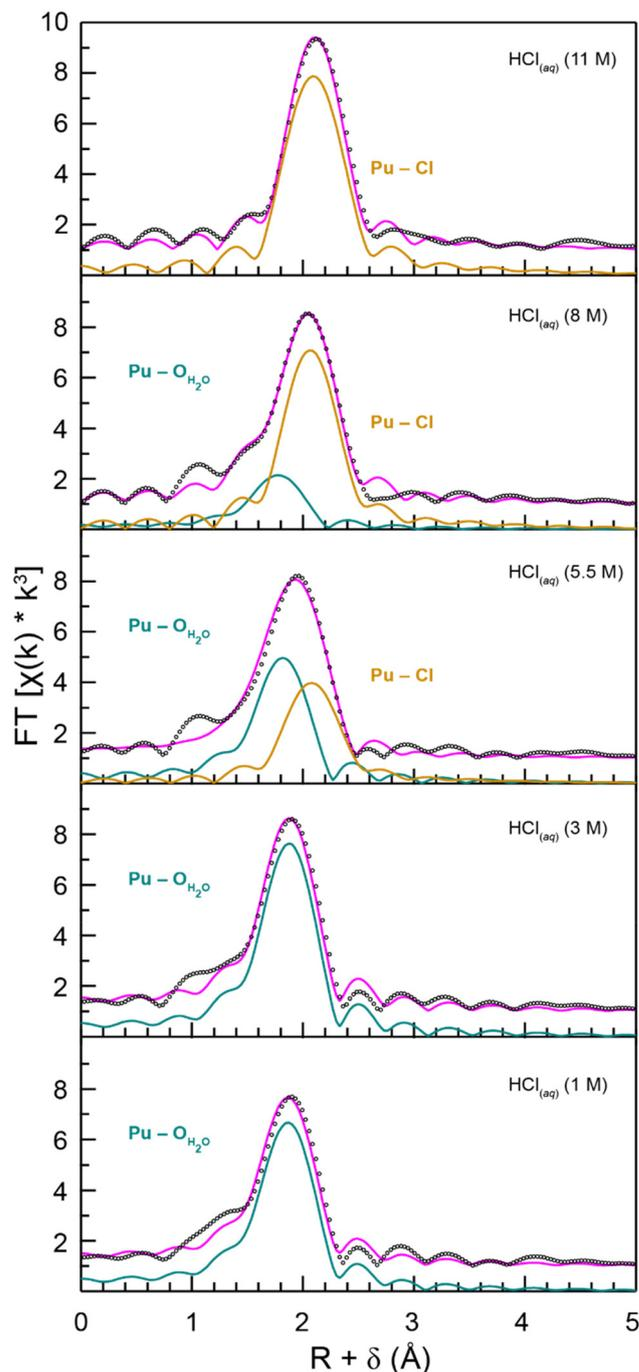
**Fig. 4** Fourier transforms of room temperature  $k^3$ -EXAFS spectra for aqueous  $\text{Pu}^{4+}_{(\text{aq})}$  solutions in  $\text{HCl}_{(\text{aq})}$  at varied concentrations (1 to 11 M; black circles). Fits for the data are shown as pink traces. The  $\text{Pu} \rightarrow \text{Cl}$  and  $\text{Pu} \rightarrow \text{O}$  scattering pathways used to generate the fits are shown as yellow and blue traces, respectively.
