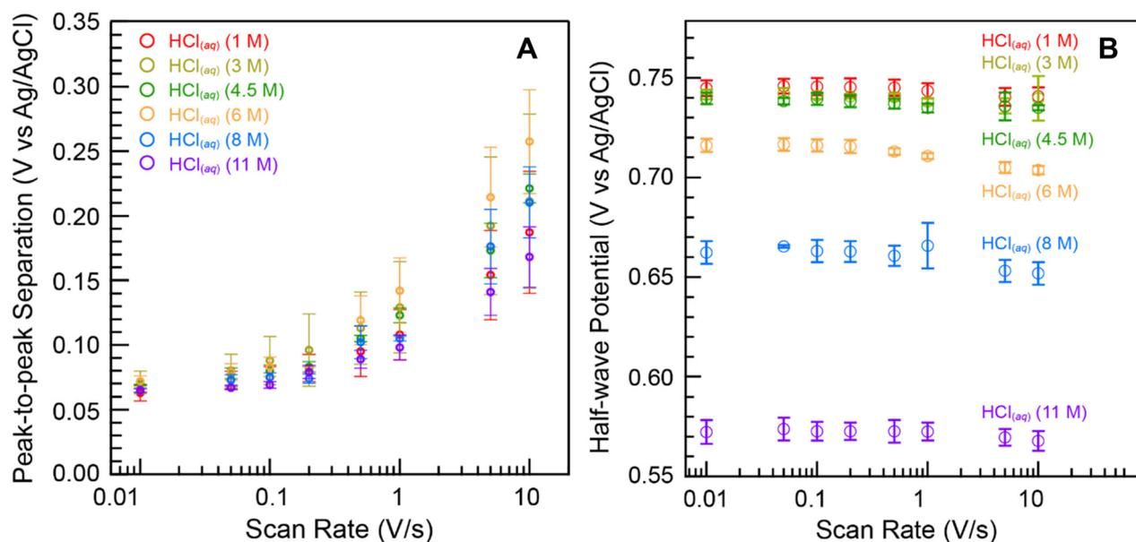
Fig. 7 (A) Cathodic and anodic peak separation potential ( $\Delta E_p$ ) and (B) half-wave potential ( $E_{1/2}$ ) as a function of the scan rate from plutonium (16.7 mM) dissolved in  $\text{HCl}_{(\text{aq})}$  (1–11 M) solutions. Error bars are the standard deviation from three replicates.
