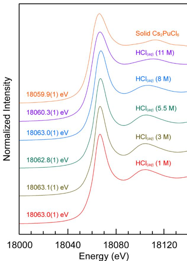
**Fig. 1** Room temperature, background-subtracted, and normalized Pu  $L_{3}$ -edge XANES spectra from  $\text{Pu}^{4+}_{(\text{aq})}$  in  $\text{HCl}_{(\text{aq})}$  solutions (1–11 M from top to bottom). The orange trace is the low temperature (77 K) background-subtracted and normalized Pu  $L_{3}$ -edge XANES spectrum from the solid  $\text{Pu}(\text{IV})$  standard ( $\text{Cs}_2\text{PuCl}_6$ ).<sup>60</sup> Inflection point energies are included.
