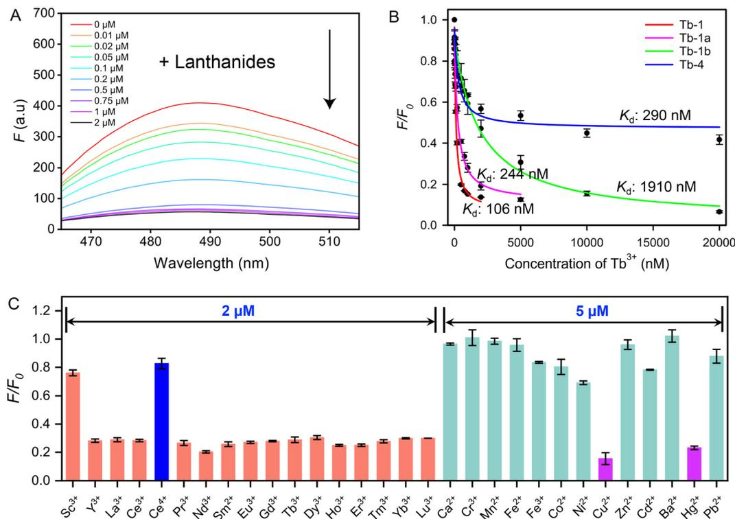
**Fig. 2** (A) Fluorescence spectra of titrating  $\text{Tb}^{3+}$  to a Tb-1/ThT mixture. (B) Titration curves of  $\text{Tb}^{3+}$  into the Tb-1 aptamer, its two mutations Tb-1a and Tb-1b, and the Tb-4 aptamer. (C) The selectivity of the Tb-1 aptamer against various metal ions using the ThT assay. The reactions were performed with 0.5  $\mu\text{M}$  aptamer, 1  $\mu\text{M}$  ThT in 10 mM MES buffer (pH 6) with 100 mM NaCl and 2 mM  $\text{MgCl}_2$ .
