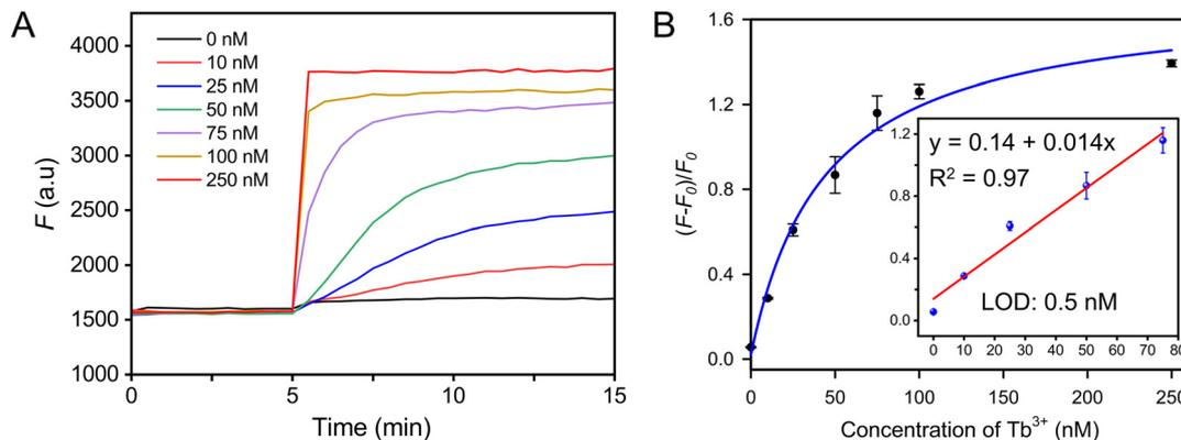
**Fig. 5** Fluorescent strand-displacement aptamer biosensor for the detection of  $Tb^{3+}$  in Lake Ontario water. (A) Kinetics traces of the 20 nM biosensor in the presence of various concentrations of  $Tb^{3+}$  in lake water. (B) The calibration curve of the sensor. Inset: linear response at low  $Tb^{3+}$  concentrations. The water contained 10 mM MES, 100 mM NaCl, and 2 mM  $MgCl_2$ , with the pH adjusted to 6.
