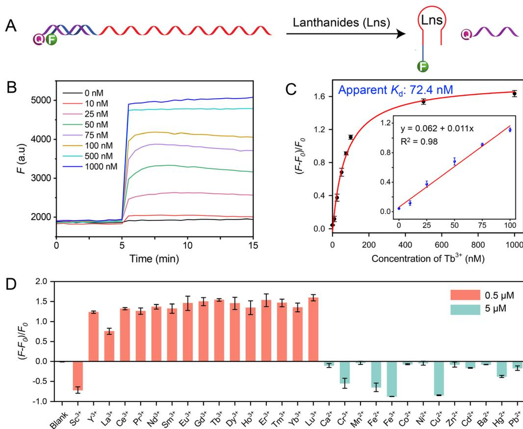
**Fig. 3** (A) A scheme of the strand-displacement biosensor featuring a covalently attached fluorophore and quencher. (B) Response of the strand-displacement biosensor to various concentrations of  $\text{Tb}^{3+}$ . (C) Calibration curves of the biosensor for  $\text{Tb}^{3+}$ . (D) The selectivity of the Tb-1 strand-displacement biosensor against various metal ions.
