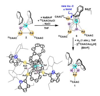
Scheme 2 Synthesis and H<sub>2</sub> reactivity of tetranuclear complex 5. The solid-state structure of 5 is provided with thermal anisotropic displacement ellipsoids displayed at the 50% probability level. BArF anion and non-hydride H-atoms are omitted for clarity. The hydride H-atoms were resolved in the Fourier map; their locations were refined freely and their  $U_{\rm iso}$  values were treated with a riding model.
