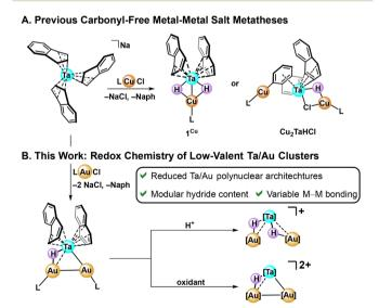
Fig. 2 Synthesis of early—late heterometallic hydride complexes *via* carbonyl-free metal—metal salt metathesis. Our prior disclosure investigated the metathesis, hydride origination, and reductive chemistry of Ta/Cu compositions (A). This work expands the chemistry to gold, showcasing the effect of oxidation and protonation state on metal—metal bonding (B).
