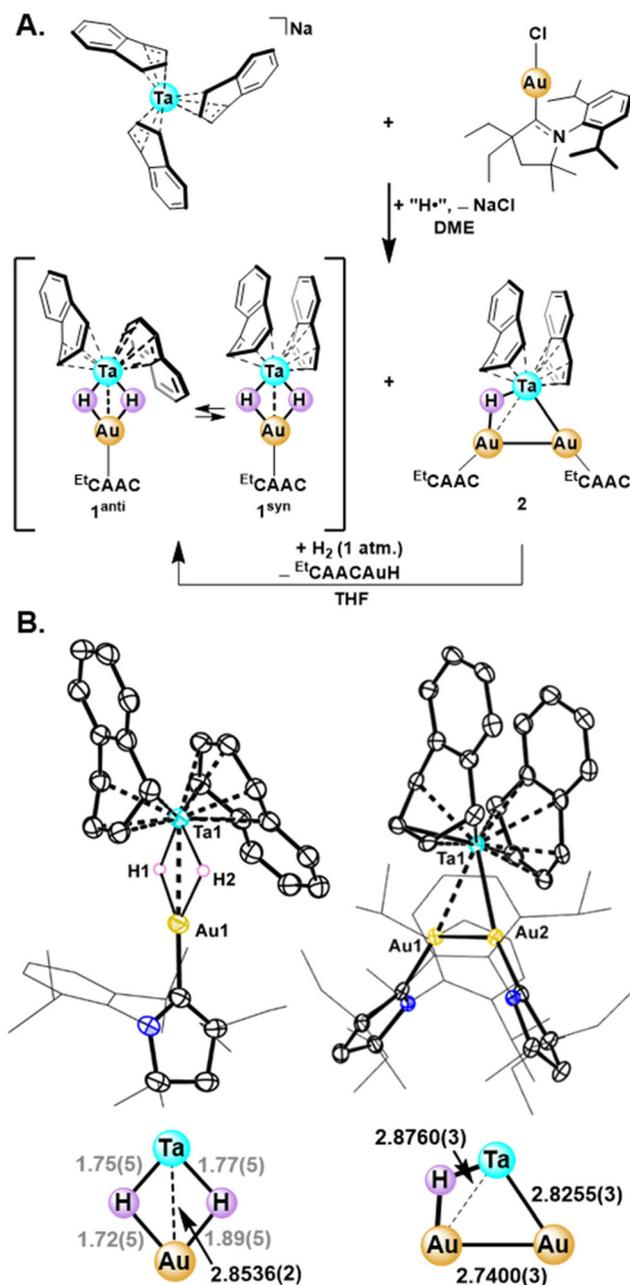
**Fig. 3** Synthetic pathway to (A) and solid-state structures of (B) mixed Ta/Au bi- and trimetallic hydride complexes. SCXRD structures are shown with thermal anisotropic displacement ellipsoids at a 50% probability level and non-hydride H atoms omitted for clarity. The hydride H-atoms in **1** were resolved in the Fourier map; their locations were refined freely and their  $U_{iso}$  values were treated with a riding model. Bond metrics for the bimetallic cores are reported in Å.
