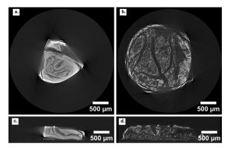
Fig. 3 XCT reconstruction slices of ceramics resulting from (a) Cu (NO<sub>3</sub>)<sub>2</sub> and (b) CuCl<sub>2</sub> infusion into concentrated hydrogels (2:1), along with their corresponding vertical cross-sections (c) and (d). The Cu (NO<sub>3</sub>)<sub>2</sub> sample displays dense regions characterized by large cracks, while the CuCl<sub>2</sub> sample reveals a foam-like structure with surface grooves.
