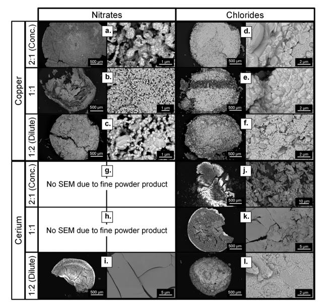
Fig. 4 SEM of Cu and Ce ceramics resulting from the HIAM process showing the impact of anions and resin formulations on the final morphology. Results from the infusion of Cu(NO<sub>3</sub>)<sub>2</sub> salt (a-c) and CuCl<sub>2</sub> salt (d-f) showed that morphology was impacted by resin condition and anion. Infusion of  $Ce(NO_3)_3$  (q-i) was only successful in dilute resin conditions, while  $CeCl_3$  infusion (j-l) showed morphological changes across resin conditions.
