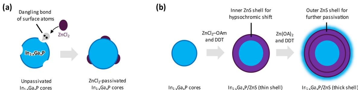
**Fig. 4** Schematic illustration of ZnS shell growth on  $\text{In}_{1-x}\text{Ga}_x\text{P}$  cores. (a) Surface defect passivation of  $\text{In}_{1-x}\text{Ga}_x\text{P}$  cores using  $\text{ZnCl}_2$ . (b) Double-step growth of the ZnS shell using  $\text{ZnCl}_2$ -OAm and  $\text{Zn(OA)}_2$ .
