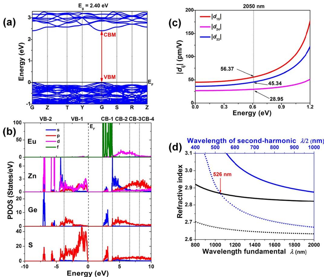
**Fig. 5** Theoretical results of electronic structures and optical parameters of  $\beta$ -EuZnGeS<sub>4</sub>: (a) band structure; (b) partial density of states; (c) calculated nonzero independent SHG coefficient  $d_{ij}$  ( $\text{pm V}^{-1}$ ); and (d) calculated refractive index dispersion curves with the shortest type-I PM cut-off wavelength.
