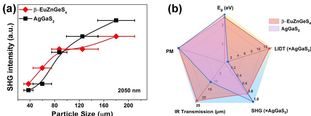
Fig. 4 (a) SHG intensities vs. particle size at  $\lambda = 2050 \text{ nm}$  for  $\beta\text{-EuZnGeS}_4$  and  $\text{AgGaS}_2$ ; (b) radar chart (five directions representing the PM feature, IR transmission, SHG, LIDT, and  $E_g$ , respectively; the colored shadows represent the areas surrounded by these optical parameters of  $\beta\text{-EuZnGeS}_4$  and  $\text{AgGaS}_2$ , respectively).
