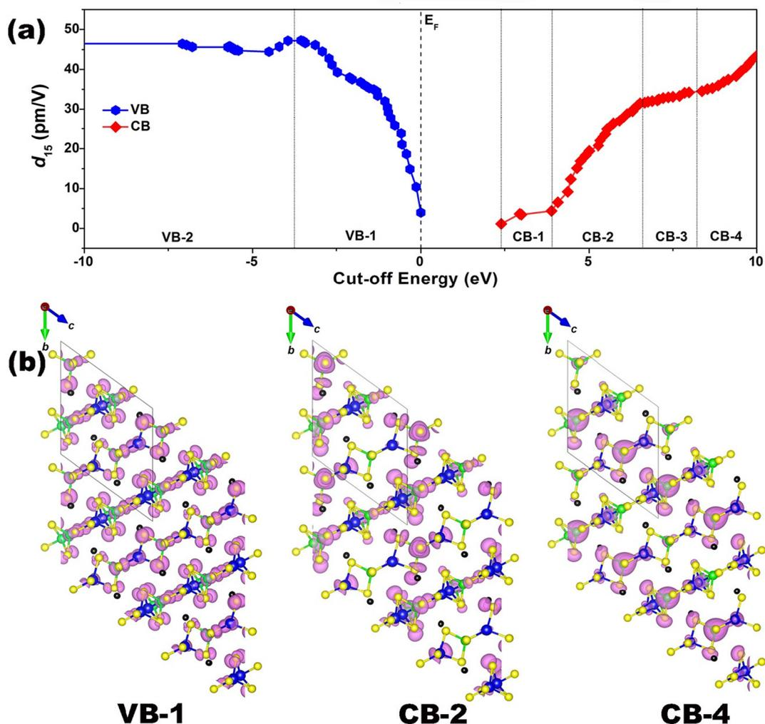
**Fig. 6** Theoretical analysis of the intrinsic mechanism of the SHG source for  $\beta$ -EuZnGeS<sub>4</sub>: (a) cut-off energy (eV) dependence of the static  $d_{15}$  (pm V<sup>-1</sup>) and (b) distribution of the partial charge density maps with major contributions in the VB-1, CB-2 and CB-4 regions. Black atoms: Eu; blue atoms: Zn; green atoms: Ge; and yellow atoms: S.
