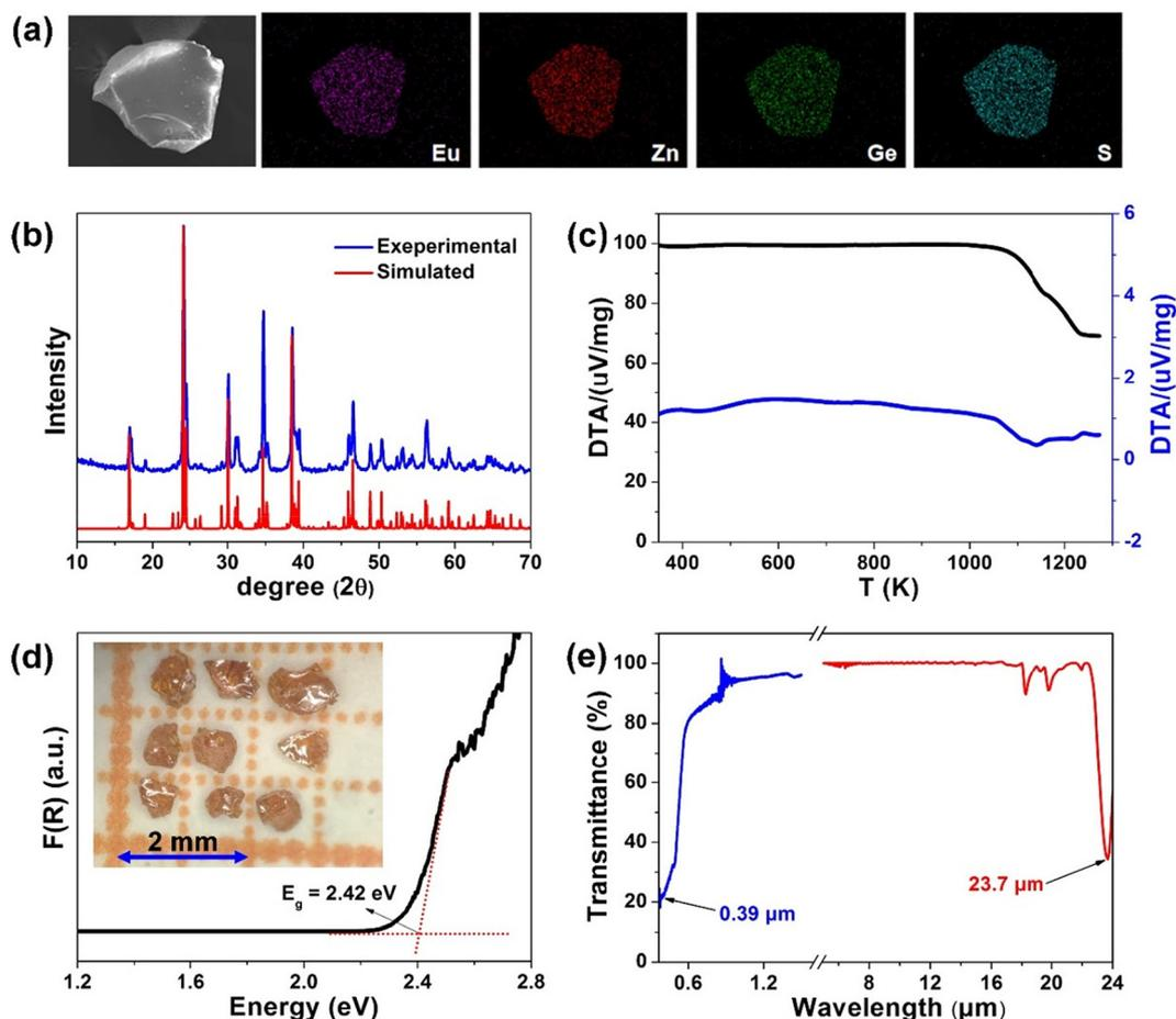
**Fig. 1** Experimental characterization results of  $\beta$ -EuZnGeS<sub>4</sub>: (a) SEM image and corresponding elemental distribution maps; (b) experimental (blue) and simulated (red) powder XRD patterns; (c) TG-DTA test curves; (d) UV-vis-NIR spectrum (inset: photograph of the title crystals); and (e) optical transmittance spectrum.
