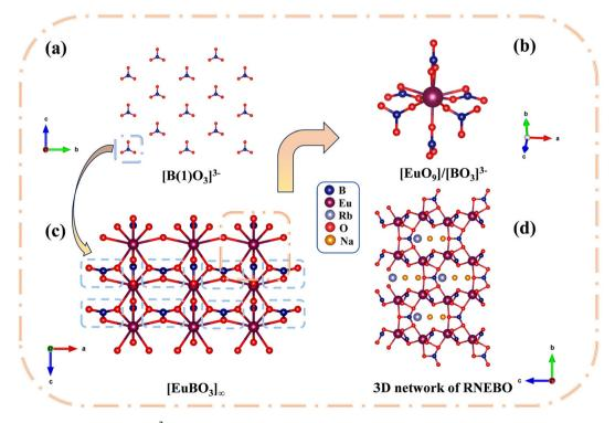
Fig. 1 (a) Coplanar arrangement of  $[B(1)O_3]^{3-}$  units between the  $[EuBO_3]_{\infty}$  layers. (b) Coordination of the  $[EuO_9]$  polyhedron with  $[BO_3]^{3-}$  units. (c)  $[EuBO_3]_{\infty}$  chains with  $[BO_3]^{3-}$  groups bridged between infinite chains along the b axis. (d) 3D network of RNEBO viewed along the a axis.
