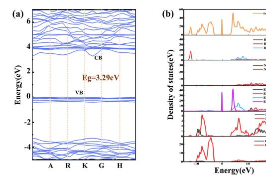
Fig. 6 (a) The electronic band structure calculated for RNEBO. (b) DOS and partial DOS projected for RNEBO.
