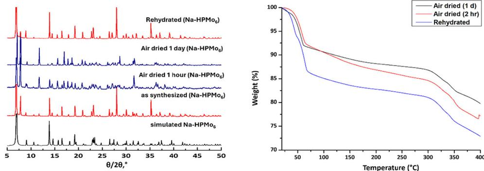
**Fig. 3** (left) Powder XRD patterns for freshly prepared, air-dried and rehydrated **Na-HPMo<sub>6</sub>** and (right) thermograms for air dried and rehydrated **Na-HPMo<sub>6</sub>** from room temperature to 400 °C under N<sub>2</sub> atmosphere.
