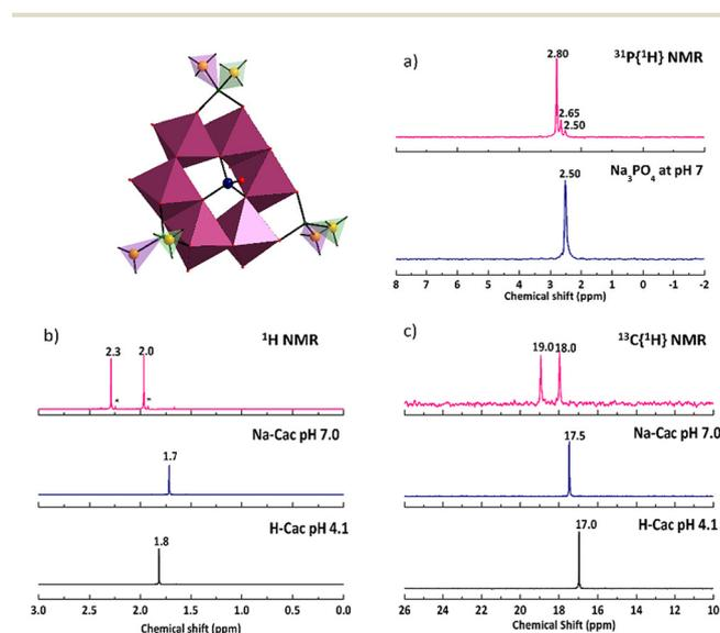
**Fig. 4** Multinuclear NMR study ((a) <sup>31</sup>P{<sup>1</sup>H}, (b) <sup>1</sup>H, (c) <sup>13</sup>C{<sup>1</sup>H}) of **NaNH<sub>4</sub>-PMo<sub>6</sub>** (pink spectra) dissolved in H<sub>2</sub>O/D<sub>2</sub>O at room temperature (pH 7). The spectra of the reference compounds are shown in blue and black.
