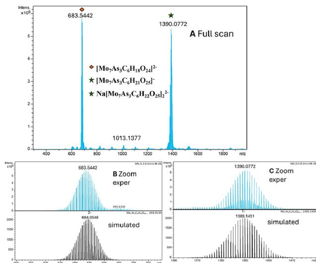
**Fig. 7** Negative mode ESI mass spectra of polyanion  $\text{Mo}_7$ . (A) Full scan full range view with two main signal clusters; (B) expanded region around  $m/z$  680 with experimental spectra in upper panel and simulated isotope pattern in bottom panel; (C) expanded region around  $m/z$  1390 with experimental spectra in upper panel (please note: signals of dimeric species at lower intensity in between main signals) and simulated isotope pattern in bottom panel.
