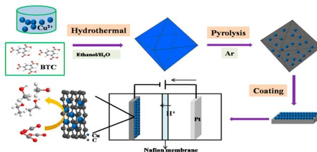
Fig. 6 Synthesis and utilization of HKUST-1-derived Cu–C composites for  $CO_2$  electroreduction to  $C_1$  and  $C_2$  alcohols. Reprinted with permission from ref. 138. Copyright 2017 American Chemical Society.
