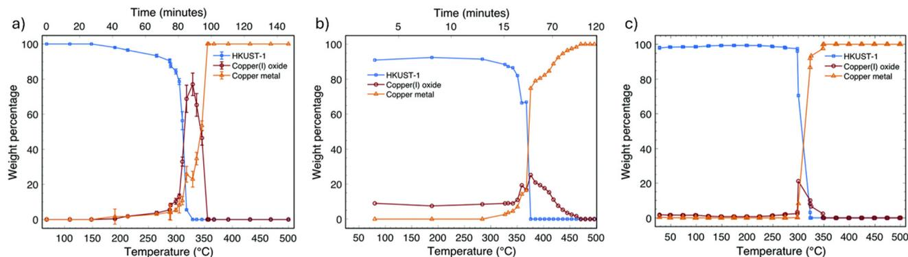
**Fig. 4** Evolution of MOF, Cu(I) oxide, and Cu(0) phases during carbonization of HKUST-1, as measured by XAS (a), X-ray PDF (b), and PXRD (c). Reproduced from ref. 96 with permission from the Royal Society of Chemistry.
