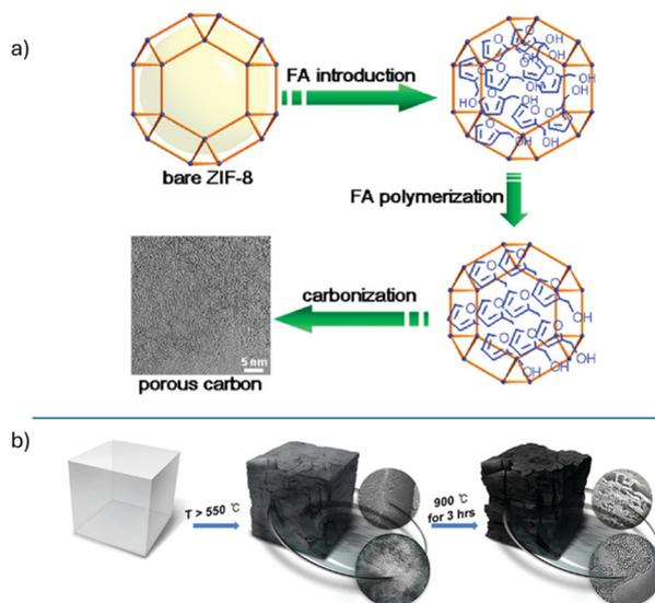
**Fig. 1** (a) Incorporation of furfuryl alcohol prior to carbonization increases carbon content in the final MOFdc material. Reprinted with permission from ref. 47. Copyright 2011 American Chemical Society; (b) direct carbonization of MOF crystals can also be achieved. Reprinted with permission from ref. 54. Copyright 2012 American Chemical Society.
