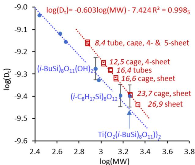
**Fig. 3**  $\log(D_t)$  vs.  $\log(\text{MW})$  for some models of MAO using  $\text{Ti}[\text{O}_2(\text{i-Bu}_8\text{Si}_8\text{O}_{11})]_2$  as a reference to construct the red calibration line. Data for POSS compounds reported in ref. 21 and 26 are shown in blue with the correlation established in ref. 26 shown as a dashed blue line.
