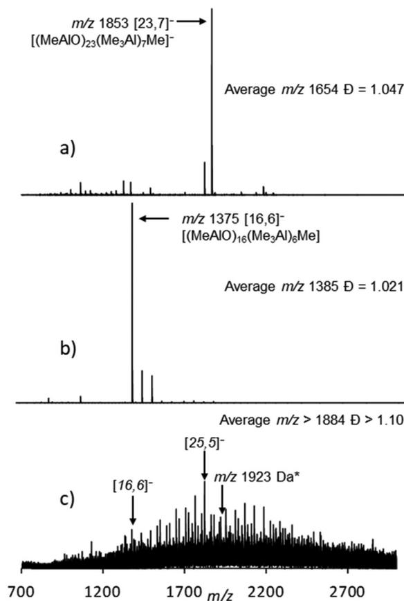
**Fig. 1** Negative ion mass spectra of hydrolytic MAO: (a) 10 wt% Sigma Aldrich, (b) 10 wt% W. R. Grace and (c) MMAO 12 (10 wt% Sigma Aldrich) in the presence of 10.0 mol% OMTS in PhF solution with  $[Al] \approx 0.01$  M. Assignments are based on MS/MS experiments and nominal mass (a and b) or just nominal mass (c). \* The peak with  $m/z$  1923 Da is assigned to the  $[(MeAlO)_{24}(n-C_8H_{17}AlO)(Me_3Al)_5Me]^-$  anion. For details, see ref. 32, 34 and 39.
