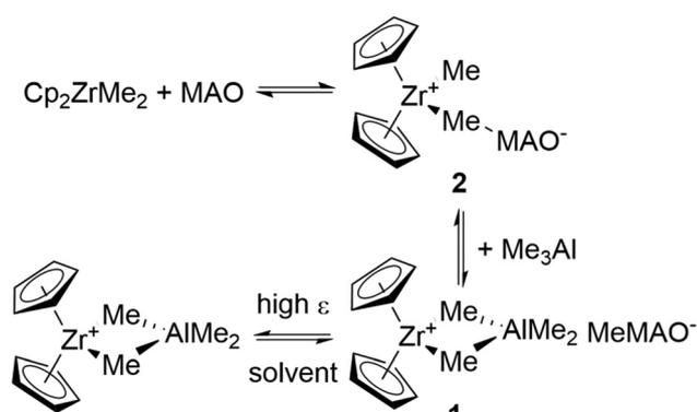
**Scheme 2** Equilibria between  $\text{Cp}_2\text{ZrMe}_2$ , MAO and inner and outer-sphere ion-pairs 2 and 1.
