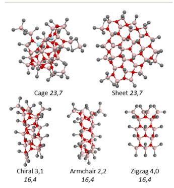
Fig. 2 Structures of some new models of MAO (Al pink, O red, C gray) with H-atoms omitted for clarity. Tetrahedral AlO<sub>4</sub> groups are highlighted in light blue for the cage 23.7 structure. For coordinate files and energies, see ESI.†
