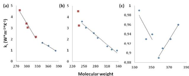
**Fig. 2** The change in thermal conductivity depending on the molecular weight of (a)  $\text{Li}_x\text{Ag}_{1-x}\text{InSe}_2$ , (b)  $\text{Li}_x\text{Ag}_{1-x}\text{GaSe}_2$  and (c)  $\text{AgGa}_y\text{In}_{1-y}\text{Se}_2$ . Solid lines are the least squares fittings of ML data and circles are experimental values. The solid solutions with a tetragonal symmetry ( $I\bar{4}2d$ ) are indicated in blue, while those with a rhombic symmetry ( $Pna2_1$ ) are indicated in red.
