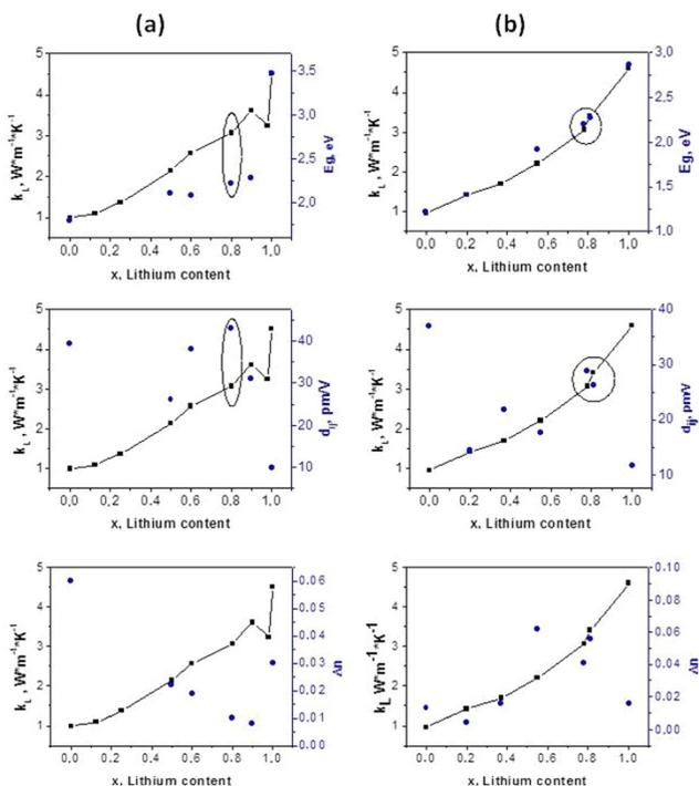
**Fig. 5** The dependence of lattice thermal conductivity ( $k_L$ ) and second harmonic generation ( $d_{ij}$ ), band gap ( $E_g$ ), birefringence ( $\Delta n$ ) on the Li content for (a) the  $\text{Li}_x\text{Ag}_{1-x}\text{GaSe}_2$  system (left column) and (b) the  $\text{Li}_x\text{Ag}_{1-x}\text{InSe}_2$  system (right column).
