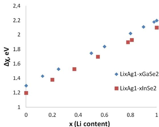
**Fig. 3** The difference in electronegativity of  $\text{Li}_x\text{Ag}_{1-x}\text{GaSe}_2$  and  $\text{Li}_x\text{Ag}_{1-x}\text{InSe}_2$  systems.
