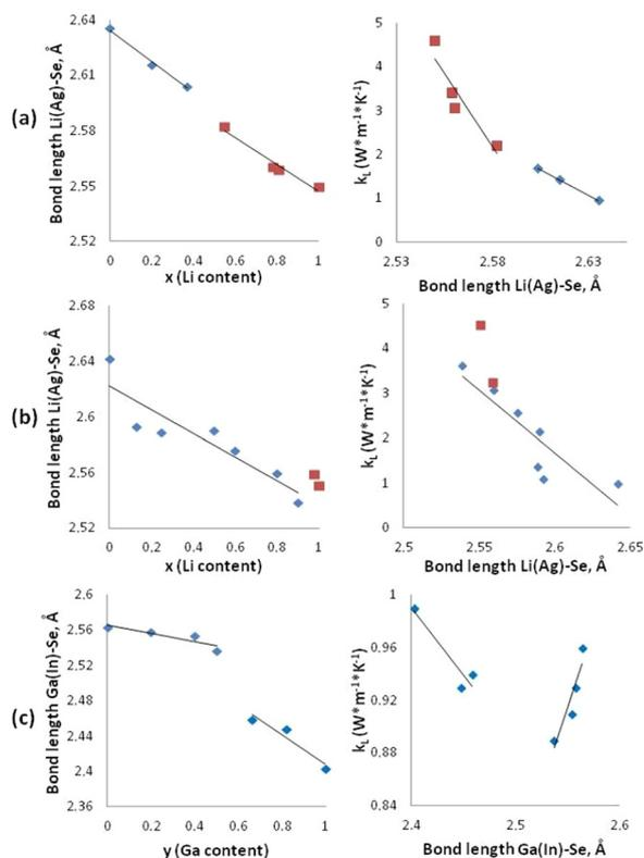
**Fig. 4** The dependence of the  $\text{Li}(\text{Ag})\text{-Se}$  bond length on the Li content and lattice thermal conductivity ( $k_L$ ) in the structures of (a)  $\text{Li}_x\text{Ag}_{1-x}\text{InSe}_2$ , (b)  $\text{Li}_x\text{Ag}_{1-x}\text{GaSe}_2$  and (c)  $\text{AgGa}_y\text{In}_{1-y}\text{Se}_2$ .
