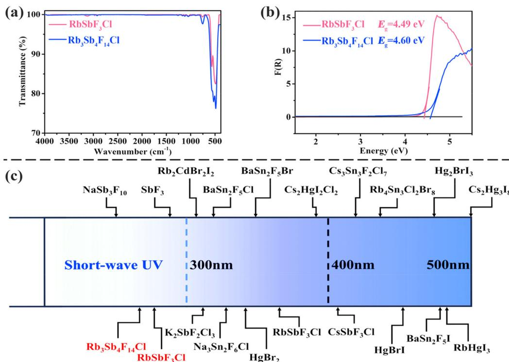
Fig. 2 (a) IR spectra of compounds RbSbF<sub>3</sub>Cl and Rb<sub>3</sub>Sb<sub>4</sub>F<sub>14</sub>Cl. (b) Band gaps for RbSbF<sub>3</sub>Cl and Rb<sub>3</sub>Sb<sub>4</sub>F<sub>14</sub>Cl. (c) Comparison of the cutoff edges of RbSbF<sub>3</sub>Cl and Rb<sub>3</sub>Sb<sub>4</sub>F<sub>14</sub>Cl with those various reported metal halides.
