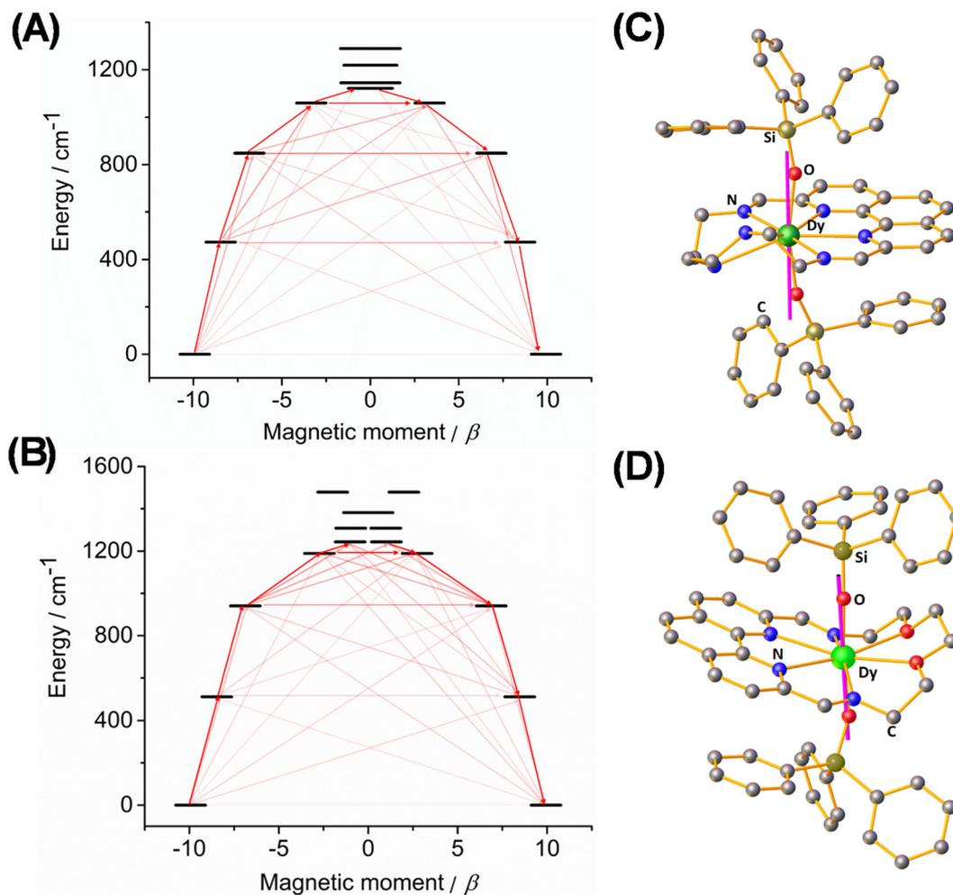
**Fig. 6** Single\_Aniso computed energy of the KDs (A and B) and orientation of the ground state anisotropic axis highlighted with purple color for  $1-L_{\text{phen}}^{\text{N6}}$  (C) and  $1-L_{\text{phen}}^{\text{N4O2}}$  (D). Dark red arrows show the most probable relaxation route and light red arrows indicate less significant but non-negligible matrix elements between different  $m_J$  states.
