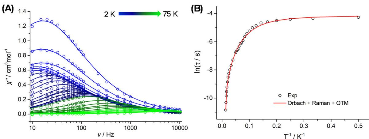
**Fig. 3** (A) Frequency-dependence of the out-of-phase ( $\chi''_{\text{M}}$ ) magnetic susceptibility under zero applied dc field over the temperature range of 2–75 K for complex  $1\text{-L}_{\text{phen}}^{\text{N6}}$ . (B) Temperature-dependence of relaxation times ( $\tau$ ) for complex  $1\text{-L}_{\text{phen}}^{\text{N6}}$ . The circles correspond to experimental data and the lines to the best-fit of the data.
