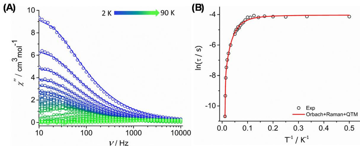
**Fig. 4** (A) Frequency-dependence of the out-of-phase ( $\chi''_M$ ) magnetic susceptibility under zero applied dc field over the temperature range of 2–90 K for complex  $1\text{-L}_{\text{phen}}^{\text{N4O2}}$ . (B) Temperature-dependence of relaxation times ( $\tau$ ) for complex  $1\text{-L}_{\text{phen}}^{\text{N4O2}}$ . The circles correspond to experimental data and the lines to the best-fit of the data.
