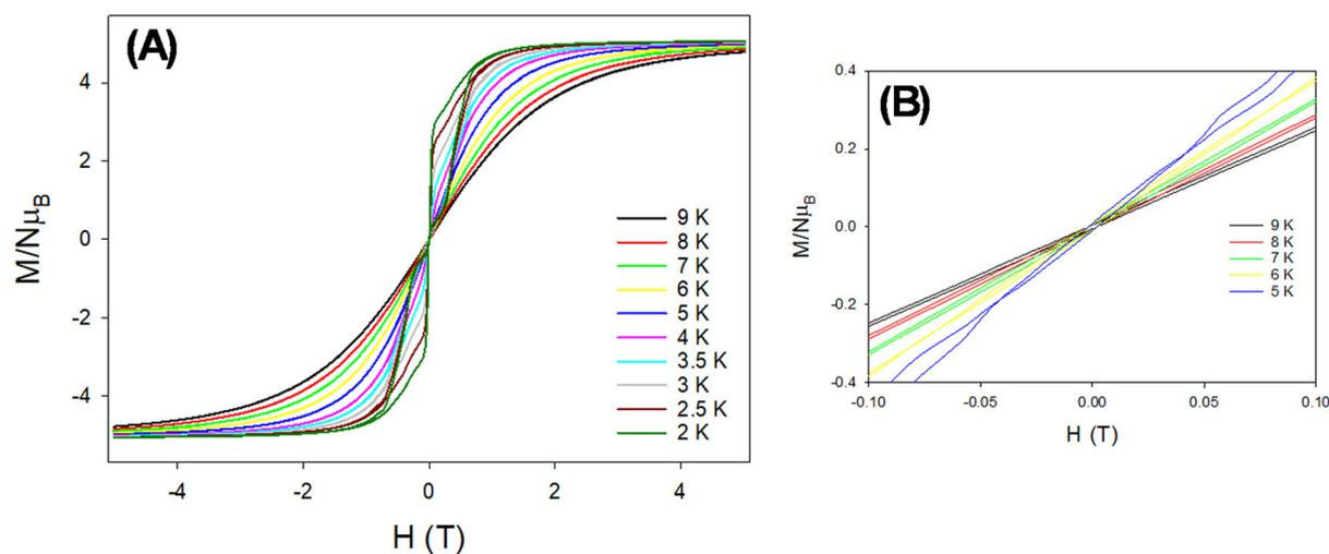
**Fig. 5** Magnetic hysteresis loops for complex  $1-L_{\text{phen}}^{\text{N4O2}}$  measured at a temperature range of 2–9 K with a mean field sweep rate of  $40 \text{ Oe s}^{-1}$  (A) and enlargement of the zero-field region from 5 to 9 K (B).
