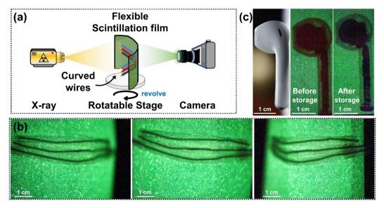
Fig. 5 (a) Schematic diagram of the flexible X-ray imaging system. (b) The X-ray radiographs of the flexible Tb-MOF-screen for curved wires (45°) with different directions. (c) The physical photograph and X-ray radiograph of the Tb-MOF-screen for the airpot before and after being stored for 60 d under ambient conditions (20-38 °C, 40-65% humidity).
