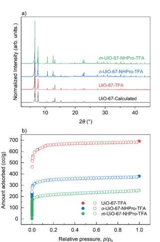
Fig. 2 (a) PXRD patterns of the as-made MOF samples with TFA as modulator; (b) nitrogen adsorption of as-made MOF samples with TFA as modulator (filled circles) and desorption (empty circles) isotherms at 77 K.
