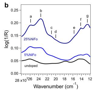
Fig. 2 (a) UV-Vis diffuse reflectance (R) spectra of undoped, 5% Co-doped, and 25% Co-doped forsterites. Groups of Co<sup>2+</sup> absorbance bands labeled a-j according to assignments of Ullrich et al.<sup>60</sup> (b) UV-Vis diffuse reflectance spectra of undoped, 5% Ni-doped, and 25% Ni-doped forsterites. Ni<sup>2+</sup> absorbance bands labeled a-g according to assignments of Hu et al.<sup>58</sup>
