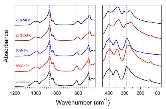
Fig. 3 ATR-FTIR spectra of synthetic forsterites in the 1200–440 cm<sup>-1</sup> range (left) and the 440–80 cm<sup>-1</sup> range: undoped forsterite (black trace), 5% and 25% Co-doped forsterite (red traces), and 5% and 25% Ni-doped forsterite (blue traces). Gray dashed lines mark peaks in the undoped forsterite spectrum. Spectra were normalized to the 871 cm<sup>-1</sup> peak.
