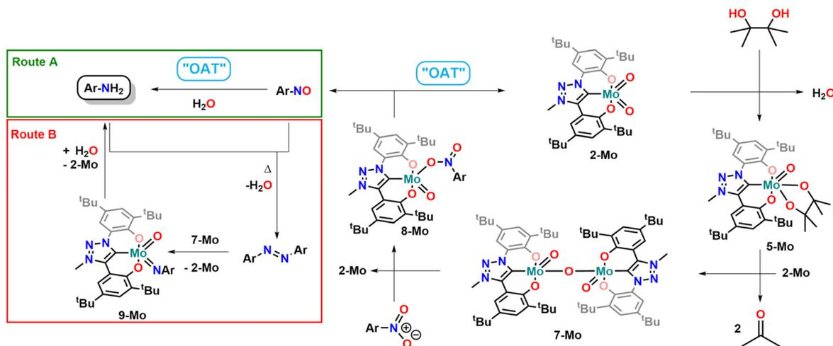
**Fig. 6** Proposed mechanism for the oxygen-atom-transfer reaction mediated by **2-Mo** in the presence of pinacol in catalytic reduction of nitroarenes (right part) and the proposed mechanism of nitrosoarene reduction *via* direct deoxygenation reaction (Route A) or *via* azoarene cleavage (Route B/left part).
