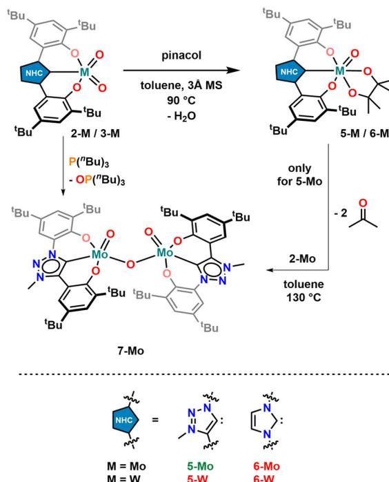
**Scheme 3** Reaction of dioxomolybdenum complexes **2-Mo/3-Mo** with pinacol to give pinacolate complex **5-Mo/6-Mo** and subsequent comproportionation reaction of **5-Mo** and **2-Mo** to the  $\mu$ -oxo bridged dimer **7-Mo**. Green labels indicate successful, red labels unsuccessful synthesis.
