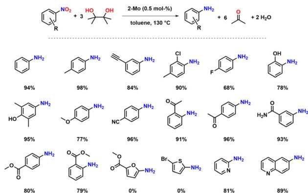
**Scheme 2** Substrate scope. Yields given correspond to isolated yields (see ESI<sup>†</sup> for further information on workup). Reactions were carried out in 10 ml J-Young tubes, using 1 mmol of substrate, 4 mmol of pinacol and the indicated amount of catalyst in 3 ml toluene.
