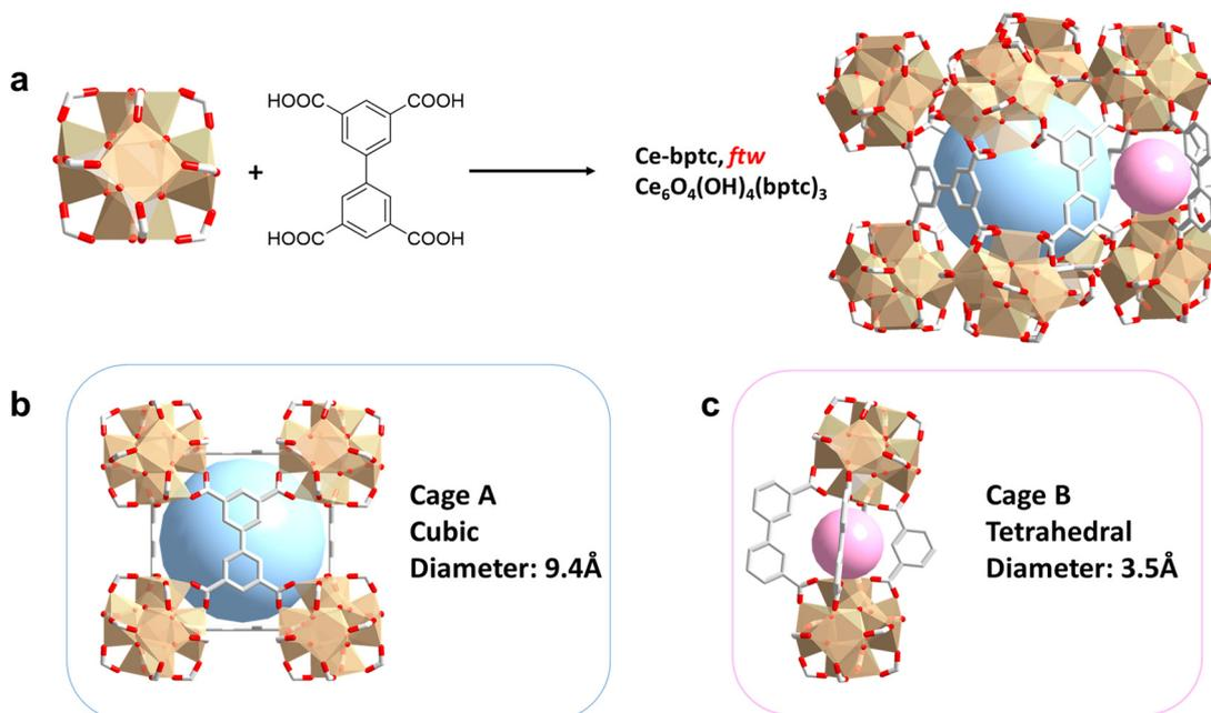
**Fig. 1** Crystal structure of Ce-bptc. (a) Views of the  $\{\text{Ce}_6\}$  cluster, linker and caged structure of Ce-bptc. (b) Detailed view of cage A (cubic cage). (c) Detailed view of cage B (tetrahedral cage). Colour code: Ce, light brown; C, grey; O, red; H, omitted for clarity. Cage A and Cage B are highlighted by blue and pink spheres, respectively.
