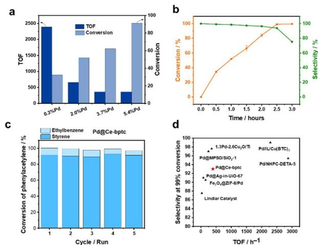
**Fig. 3** Studies of catalytic performance. Reaction conditions: 5 mg of MOF catalyst, 1 mmol of phenylacetylene, 1 mmol of mesitylene, 2 mL of THF, 25 °C, 2.5 h. (a) Conversion of phenylacetylene and selectivity for styrene on Pd@Ce-bptc at different Pd loadings. (b) Conversion of phenylacetylene and selectivity for styrene on Pd@Ce-bptc-2.0% over time. (c) Recycling test for Pd@Ce-bptc. (d) Comparison of the catalytic performance of different Pd-loaded catalysts under 1 bar H<sub>2</sub>.
