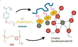
Structure and dynamics in poly(ethylene oxide)-blended single-ion conducting polymer electrolytes based on side-chain ionomers
