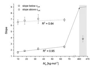
**Fig. 6** The slopes of the linear fits describing the concentration dependence of viscosity as a function of polymer molecular weight (a star represents the value for solutions of star-like polymers). The grey column shows the theoretical slope value for a linear polymer with a molar mass corresponding to that of the star-like polymer.
