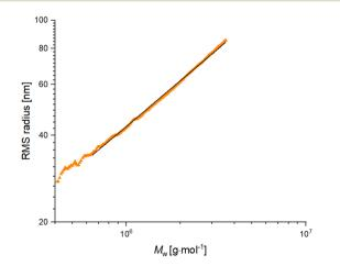
**Fig. 2** Conformation plot showing the dependence of the RMS radius of linear HPMA-based homopolymers on molecular weight. Orange – curve from the MALS detector; black – the fitted curve.
