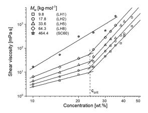
Concentration dependence of shear viscosity for polymer solutions with different molecular weights (the straight lines are linear fits of the experimental values on a log-log scale).
