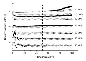
Fig. 4 Flow curves of polymer solutions with  $M_{\rm w} = 64.3$  kg mol<sup>-1</sup> at 25 °C at various solution concentrations (10-35 wt%). Experiments were performed in duplicates (empty and filled marks).
