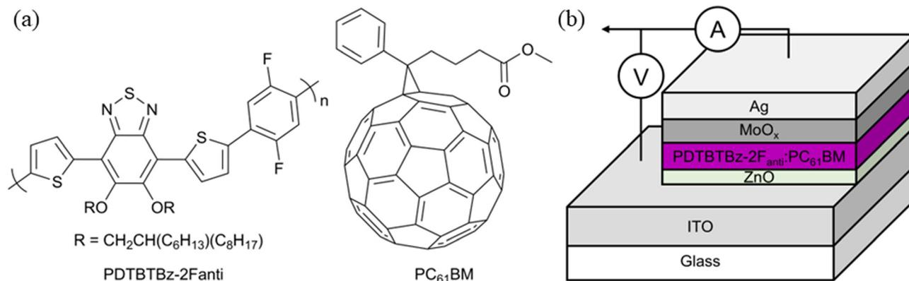
**Fig. 5** (a) Chemical structures of PDTBTBz-2F<sub>anti</sub> and PC<sub>61</sub>BM fullerene derivative used in the BHJ of the OSCs; (b) schematic representation of the complete bulk heterojunction solar cell device architecture showing the different layers: glass substrate, ITO electrode, ZnO electron transport layer, PDTBTBz-2F<sub>anti</sub>:PC<sub>61</sub>BM active layer, MoO<sub>x</sub> hole transport layer, and silver top electrode.
