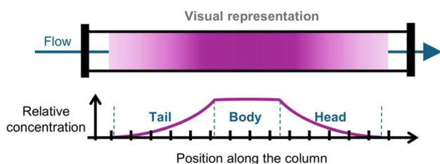
**Fig. 7** Representation of the dilution effect during continuous flow synthesis in a column reactor: (top) visual representation of the concentration gradient within the column; (bottom) corresponding relative concentration profile showing the characteristic tail, body, and head regions of the reaction mixture along the column length.
