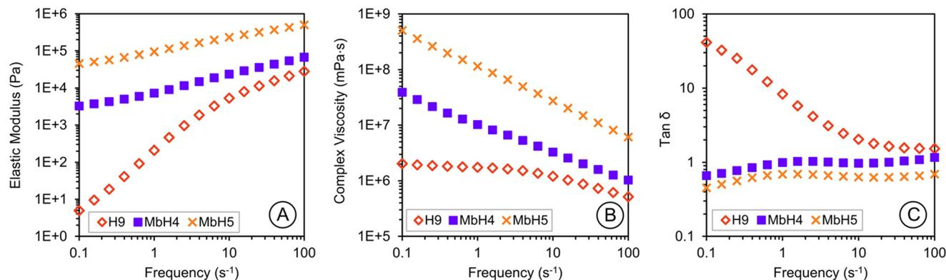
**Fig. 6** Frequency sweep results using a fixed 0.1% strain for diblock p(MMA-*b*-DHIAMA) contrasted with p(DHIAMA) homopolymer at 25 °C: (A) elastic modulus; (B) complex viscosity; and (C)  $\tan \delta$ .
