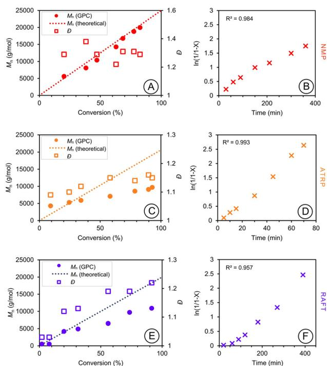
Fig. 2 RDRP reaction kinetics for DHIAMA: number average molecular weight ( $M_n$ ) by GPC, calculated theoretical  $M_n$ , and dispersity ( $D$ ) throughout polymerization by: (A) NMP; (C) ATRP; and (E) RAFT. Linearized monomer conversion (semi-logarithmic) during polymerization is shown by: (B) NMP; (D) ATRP; and (F) RAFT. Reaction conditions are provided in section 2.1.
