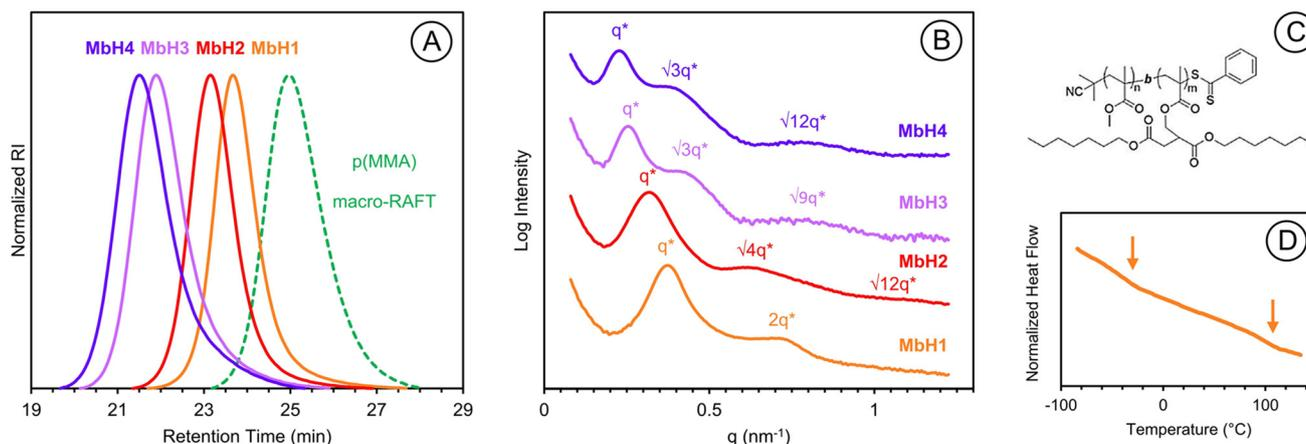
**Fig. 5** Diblock copolymer characterization: (A) GPC traces of macro-RAFT agent and final p(MMA-*b*-DHIAMA) diblock polymers; (B) SAXS spectra of the p(MMA-*b*-DHIAMA) series indicating the presence of microdomains; (C) schematic of p(MMA-*b*-DHIAMA) polymer; and (D) differential scanning calorimetry trace of MbH1 presenting two  $T_g$ s corresponding to the  $T_g$ s of the homopolymers.
