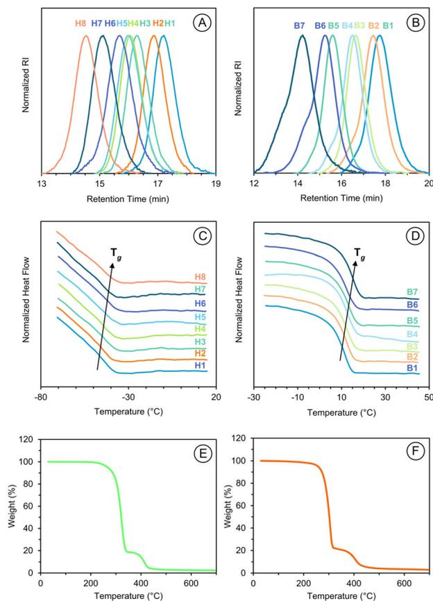
**Fig. 3** GPC traces of (A) p(DHIAMA) homopolymer series and (B) p(DBIAMA) homopolymer series. DSC traces of (C) p(DHIAMA) homopolymer series and (D) p(DBIAMA) homopolymer series. TGA trace for (E) p(DHIAMA) (H7) and (F) p(DBIAMA) (B4).
